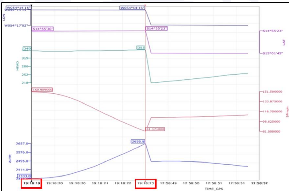
Figure 14 - DGPS data at the beginning of the change to a climb attitude (“recovery”) of the aircraft.
