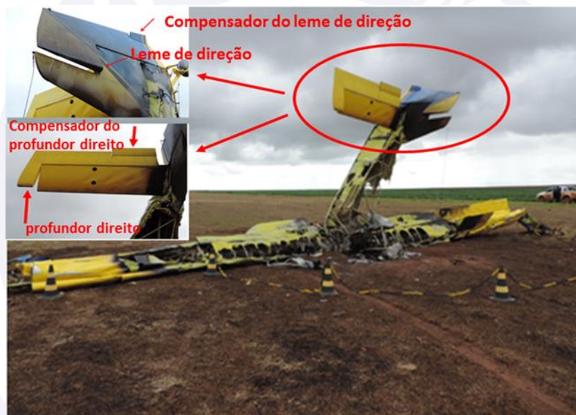
Figure 2 - Position of the command, control and trim surfaces.
