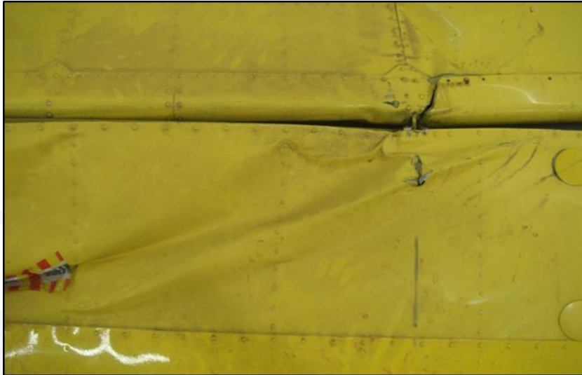
Figure 5 - Plastic deformation on the left horizontal stabilizer surface.
