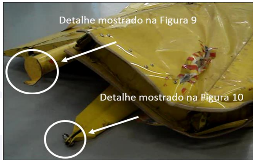
Figure 8 - End of the brace strut that was fixed to the aircraft structure.
