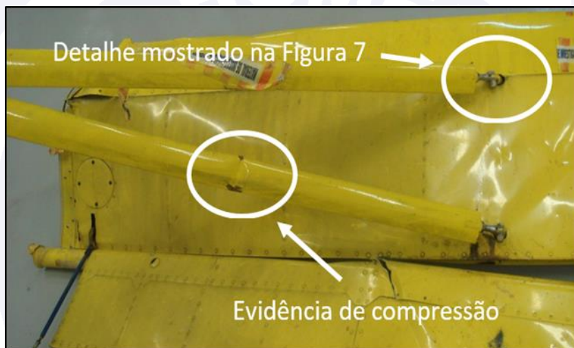
Figure 6 - Overview of the brace strut and compression strain.
