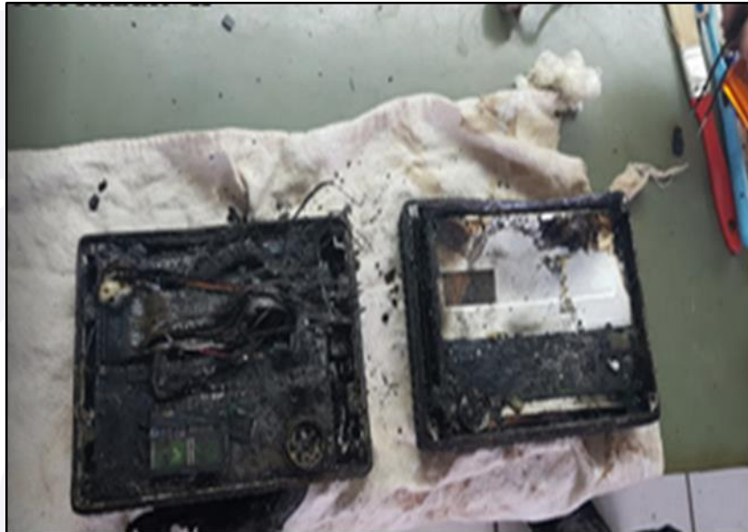
Figure 12 - Physical conditions of the DGPS that equipped the PR-AJF aircraft upon its opening in a specialized laboratory.
