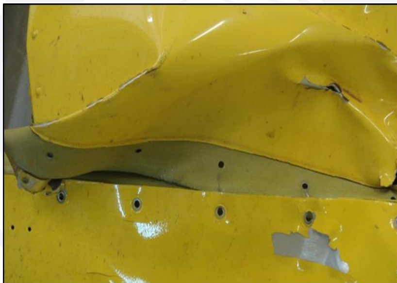
Figure 4 - Loss of rivets on the left horizontal stabilizer surface.
