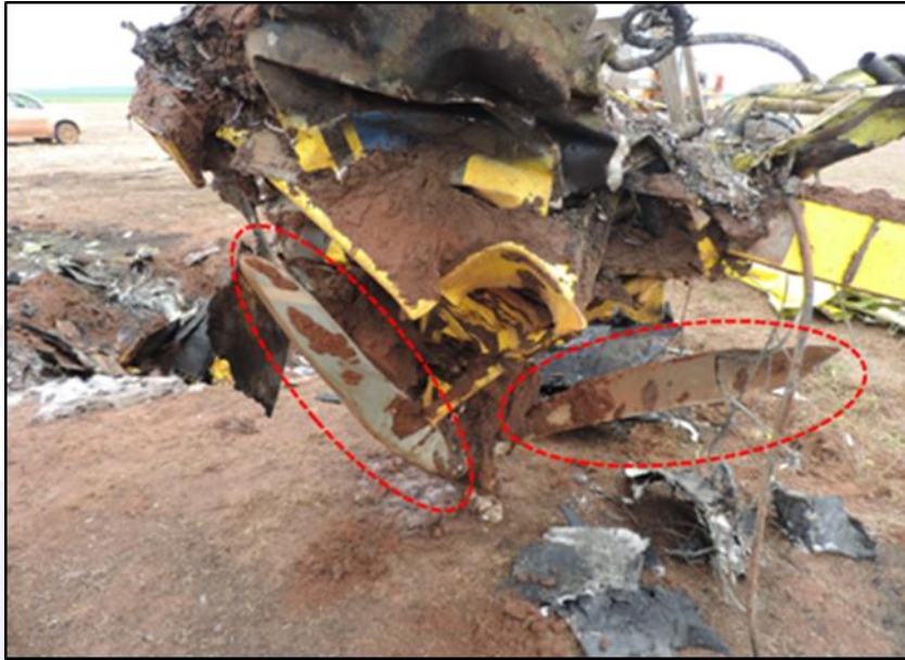
Figure 3 - Degree of the powertrain destruction and, in particular, only two of the three propeller blades.
