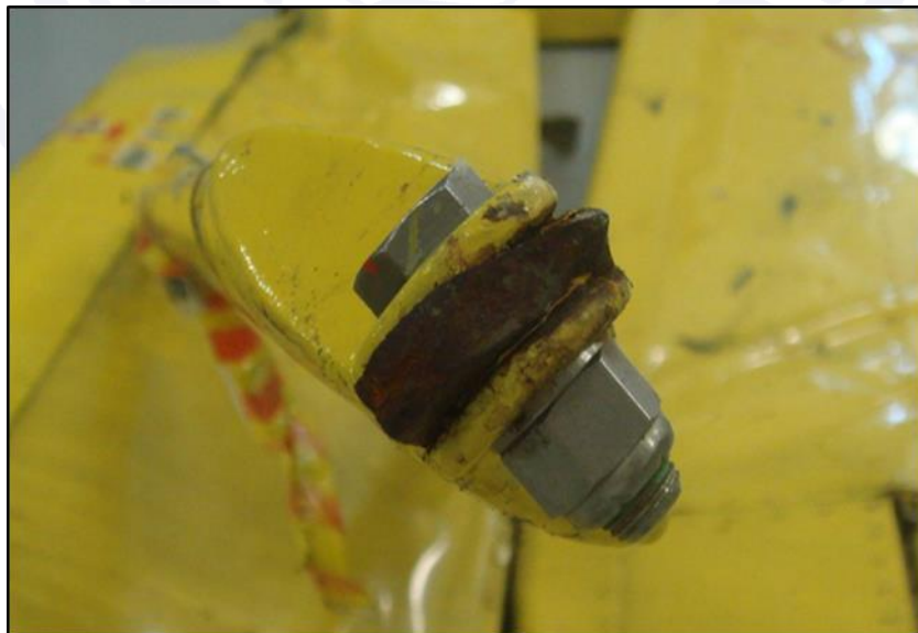
Figure 10 - Fracture surface with overload characteristic (Detail of Figure 8).
