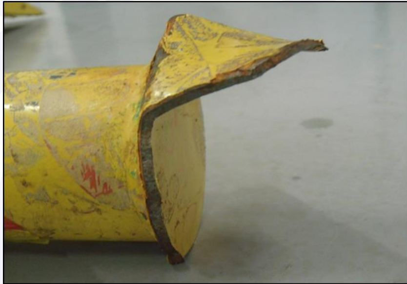
Figure 9 - Surface with typical characteristics of structure overload fracture (Detail of Figure 8).
