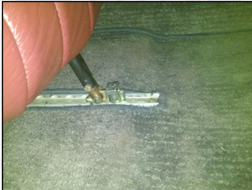
Figure 7 - Aspect of the seats assembly in the floor of the aircraft, in a similar model to the CA-9.
