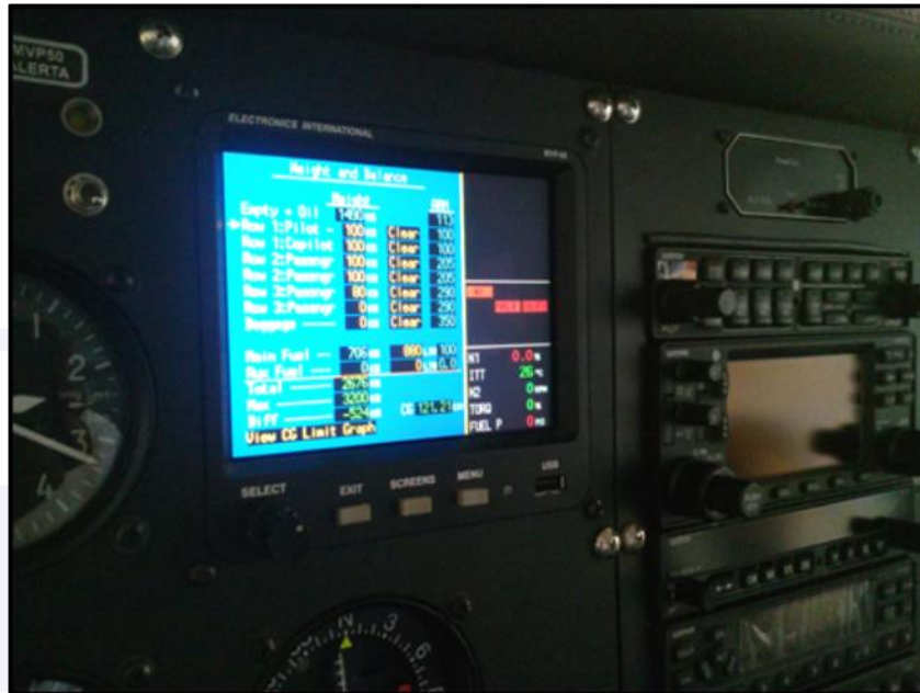
Figure 6 – Aircraft's loading warning system, installed in another aircraft model of the Kit's manufacturer.
