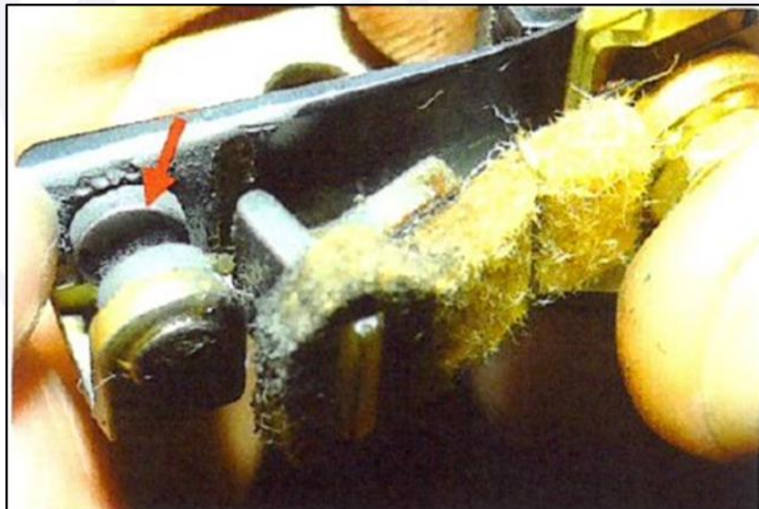
Figure 12 – Charring observed on the breaker points of the engine left magneto.
