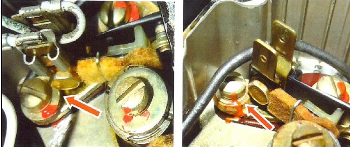
Figure 13 - Comparison between the assembly of the screw securing the electrical terminals of the engine right magneto (non-standard washer) and another similar magneto (correct washer).
