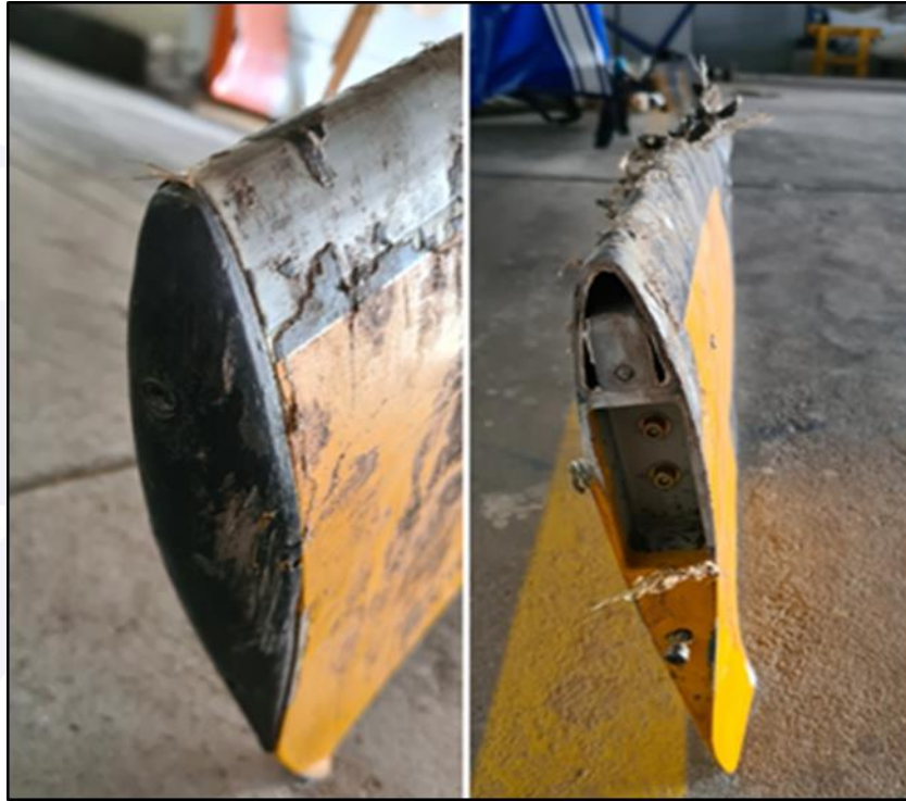
Figure 3 - View of the tips of the main rotor blades with one of them showing damage from the impact against the tail boom.
