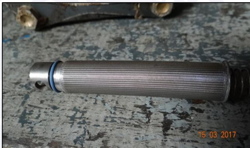
Figure 15 - View of the fuel filter at the inlet of the servo injector, with no contaminants.
