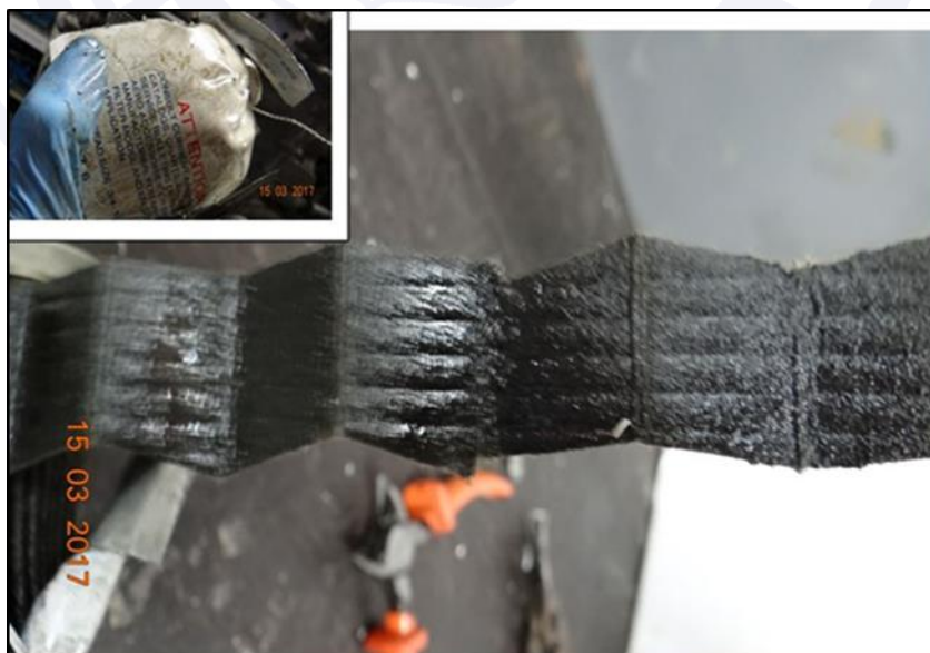
Figure 19 – Oil Filtering element with no filings. Highlighted the oil filter before opening.
