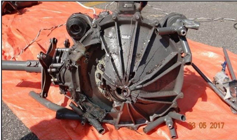
Figure 36 - View of the transmission case crankcase fracture.
