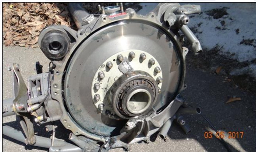
Figure 39 - Bottom view of the rack and bearing of the transmission box.
