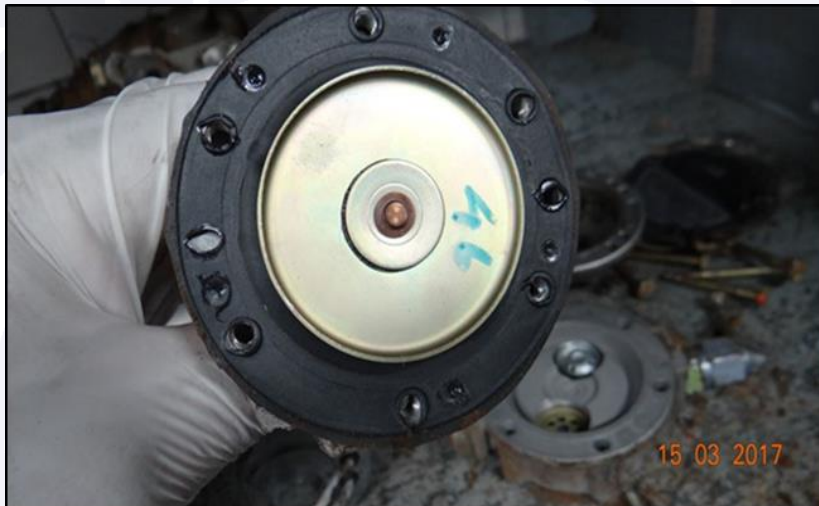
Figure 18 - Clean fuel pump diaphragm view.
