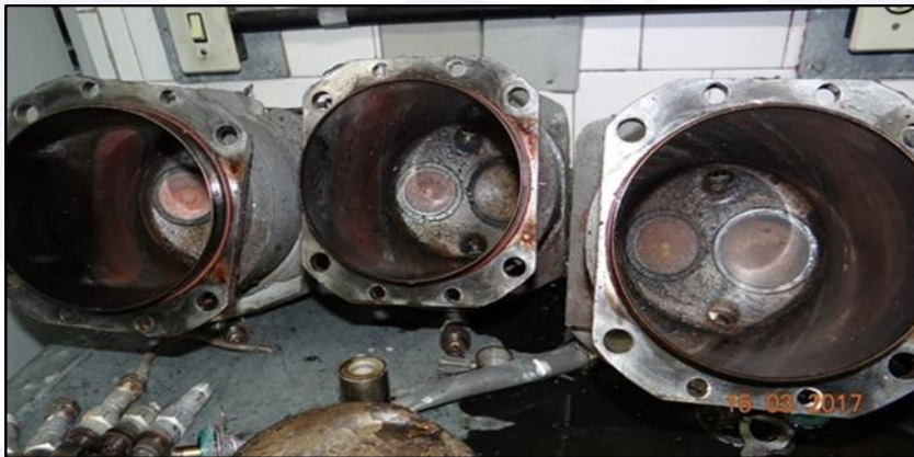
Figure 24 - View of cylinders 1, 2 and 3, with no operational damage.
