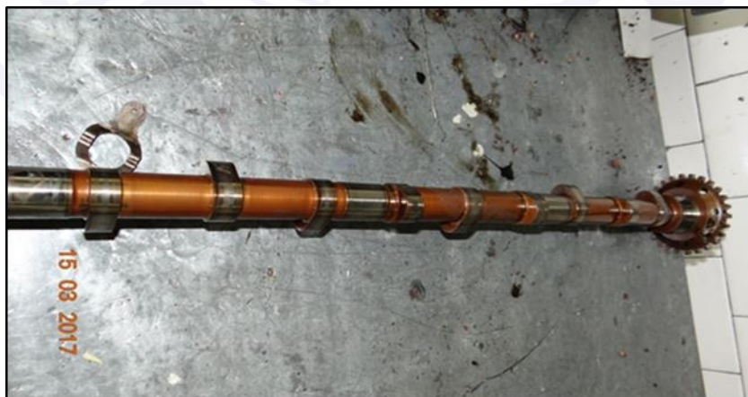
Figure 28 - Overview of the engine valve control shaft.
