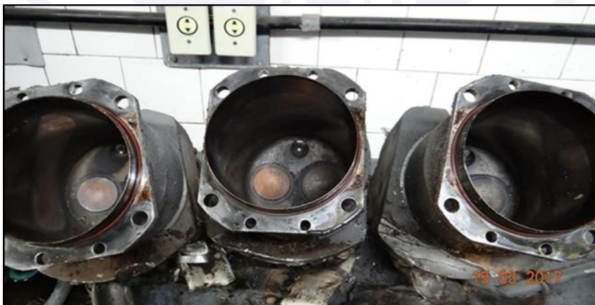
Figure 25 - View of cylinders 4, 5 and 6, without operational damage.
