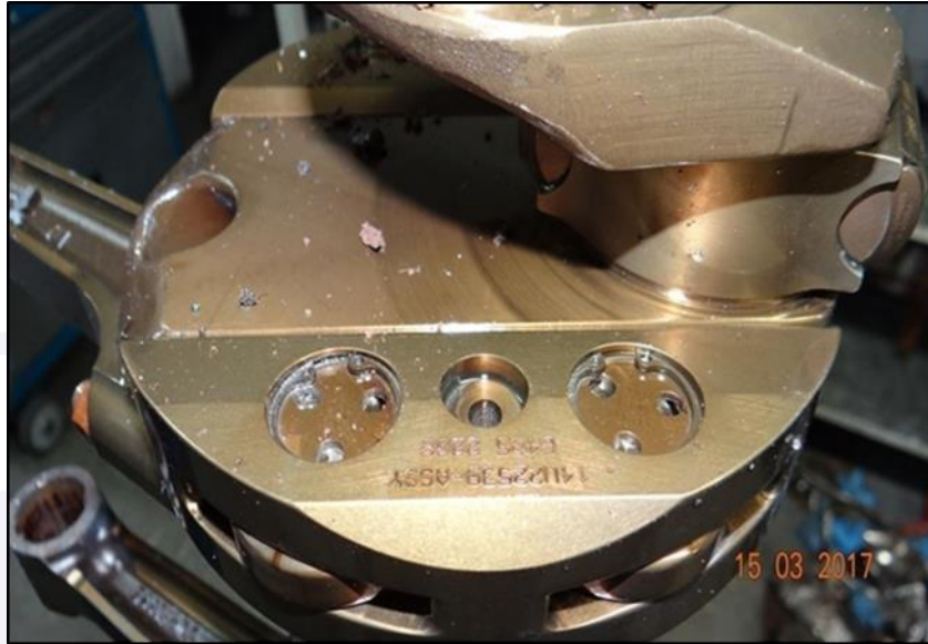
Figure 29 - Highlight for identification of the counterweight of the crankshaft.
