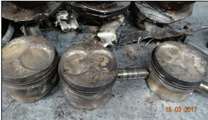
Figure 27 - View of the pistons 4, 5 and 6, with normal working color.
