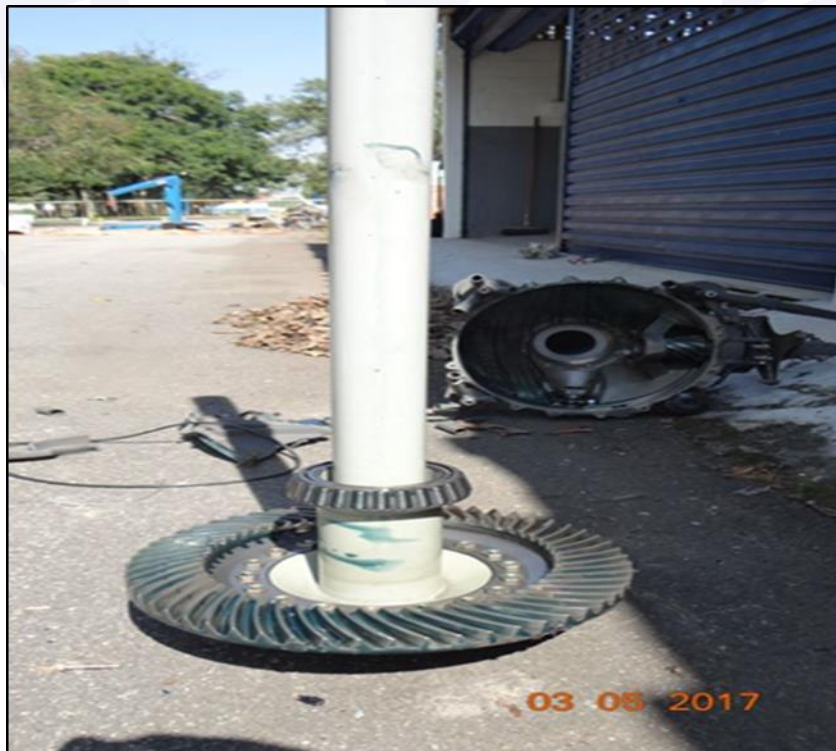
Figure 43 - Top rack and top bearing of the main gearbox.
