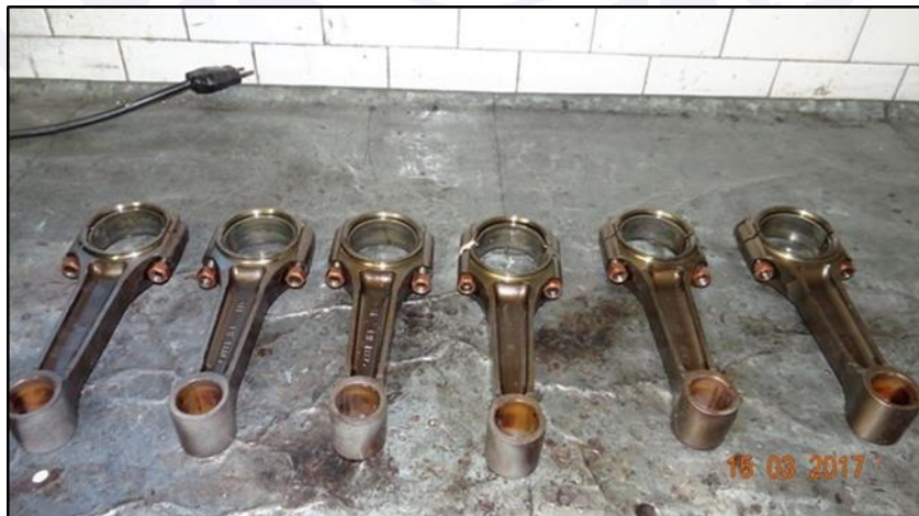
Figure 31 - View of the connecting rods in good condition.
