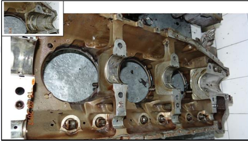
Figure 32 - View of the right semi-engine housing and of the connecting rod in good condition.
