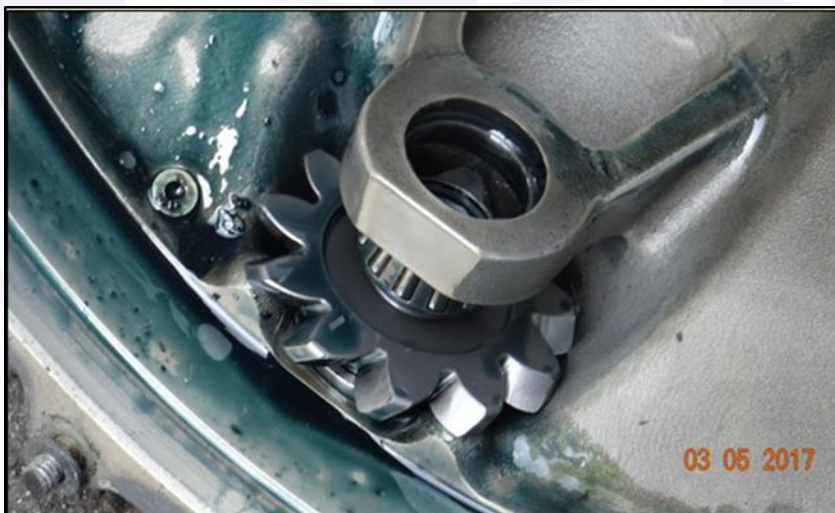
Figure 46 - Gearbox hydraulic pump drive gear.
