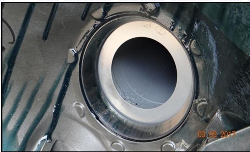
Figure 45 - External track of the upper gearbox bearing.
