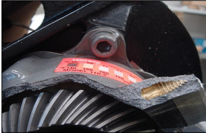
Figure 8 - Surface of fracture with aspect of overload.
