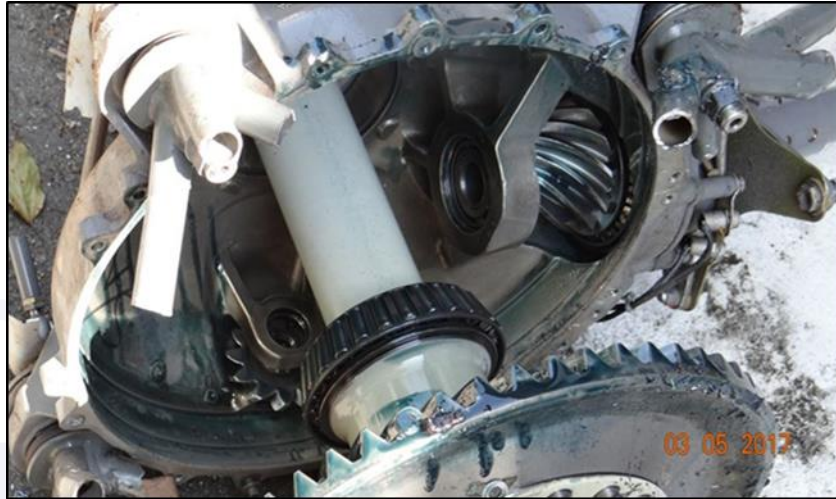
Figure 41 - General view of the rack, the upper bearing and the gearbox pinion.
