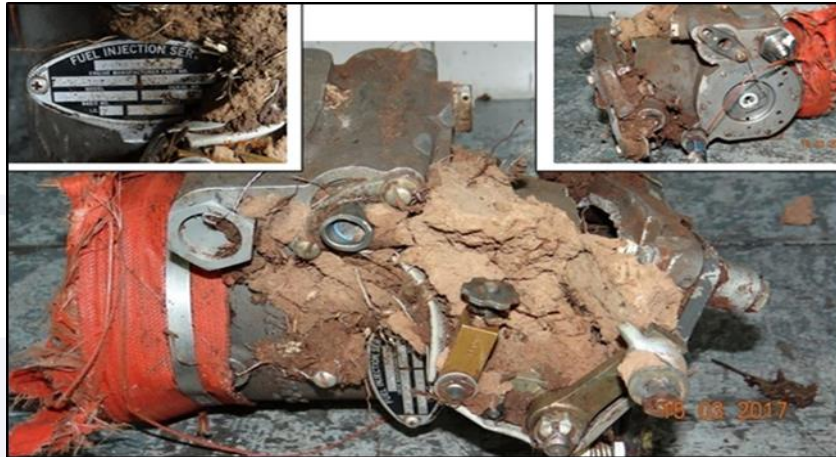
Figure 14 - Overview of the servo fuel injector. The highlights show their identification and the damages resulting from the accident.
