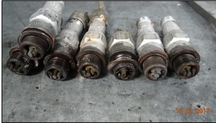
Figure 11 - Spark plugs with normal operating color.
