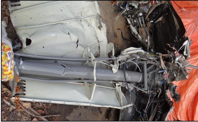
Figure 35 - Overview of the transmission assembly after opening the fairing.
