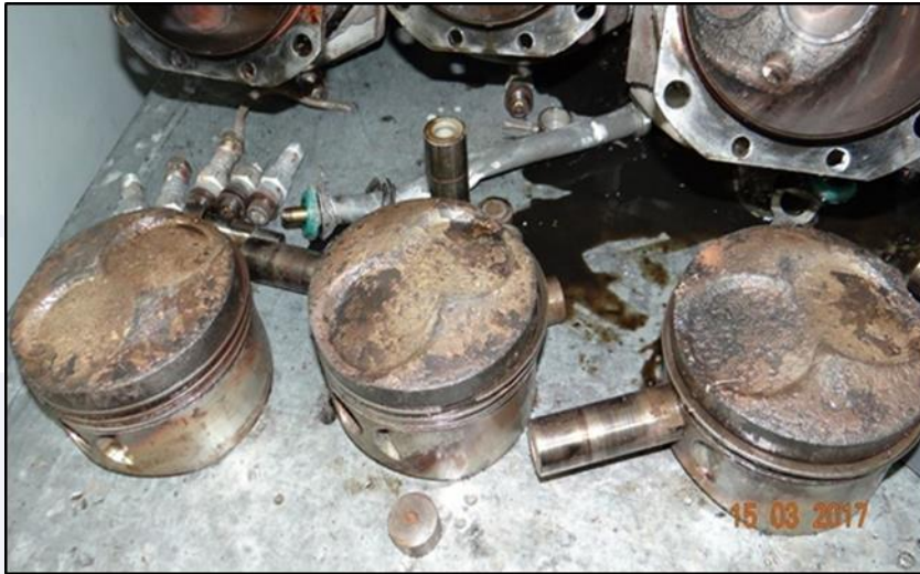
Figure 26 - View of the pistons 1, 2 and 3, with normal working color.
