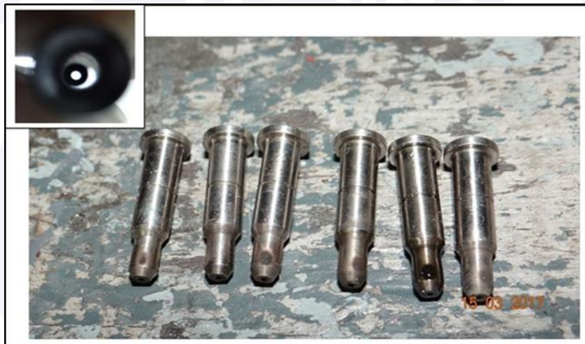
Figure 12 - View of the nozzles. Highlights the clearing.
