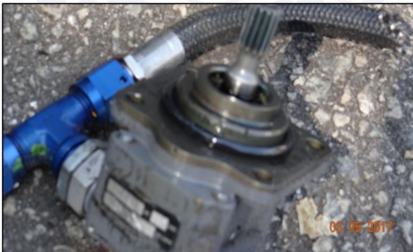
Figure 37 - Main gearbox hydraulic pump.
