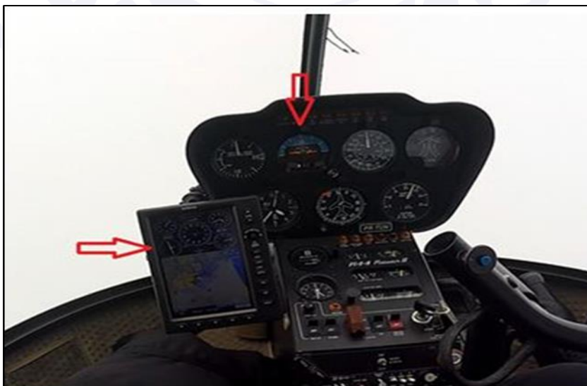
Figure 59 - 18:29:40 (UTC), aircraft attitude indicator and GPS with different indications.
