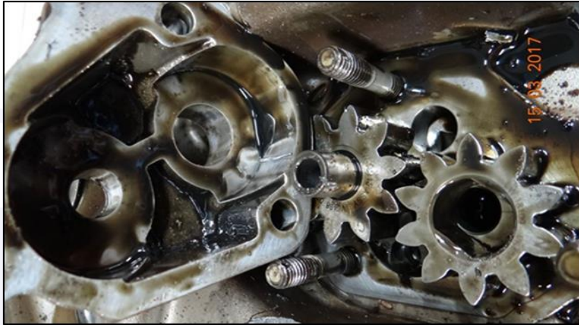
Figure 20 - Gears and housing of the engine oil pump without scratches.
