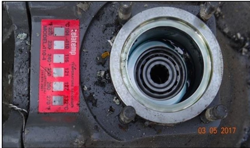
Figure 38 - Housing of the hydraulic pump in the gearbox.
