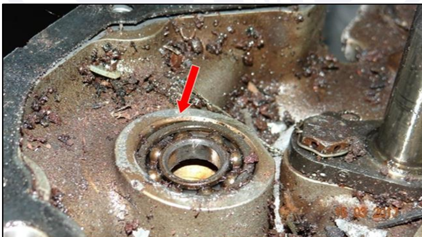
Figure 22 - Misalignment in the drive gear bearing of the right magneto.
