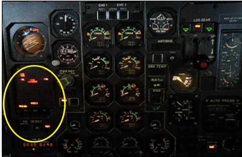
Figure 25 - Indications shown on the aircraft panel after the occurrence (highlighted).
