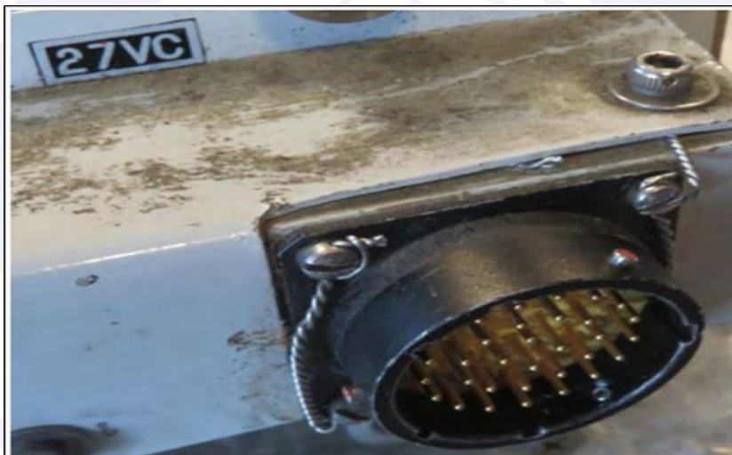
Figure 27 - Brake Wire placed inside the housing and connector in a different pattern than expected.
