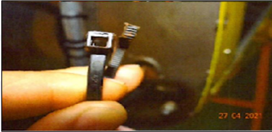
Figure 3 - Plastic clamp found on the engine cradle with the broken latch.
