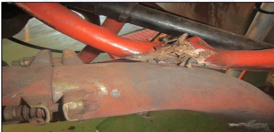
Figure 2 - Damaged engine electrical wiring, leaning against the exhaust.
