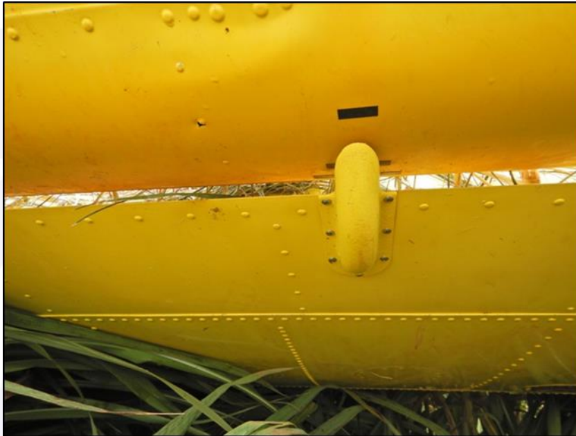
Figure 3 - Indication of the position of the flaps, at the accident site, in an intermediate position between 10° and 20°.
