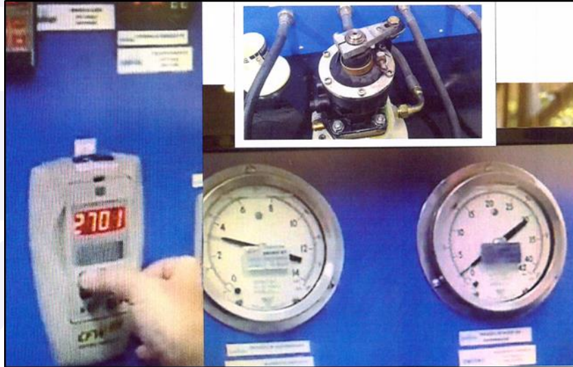
Figure 5 - Propeller governor test at 2,700 RPM. The pressure gauge on the right-hand side indicated normal internal leakage.
