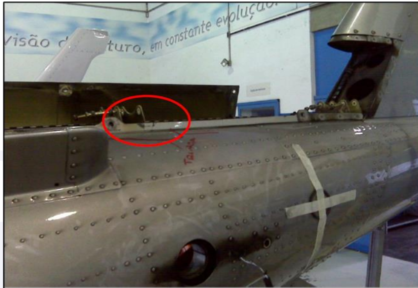
Figure 2 - Tail Boom region where the crack was found.
