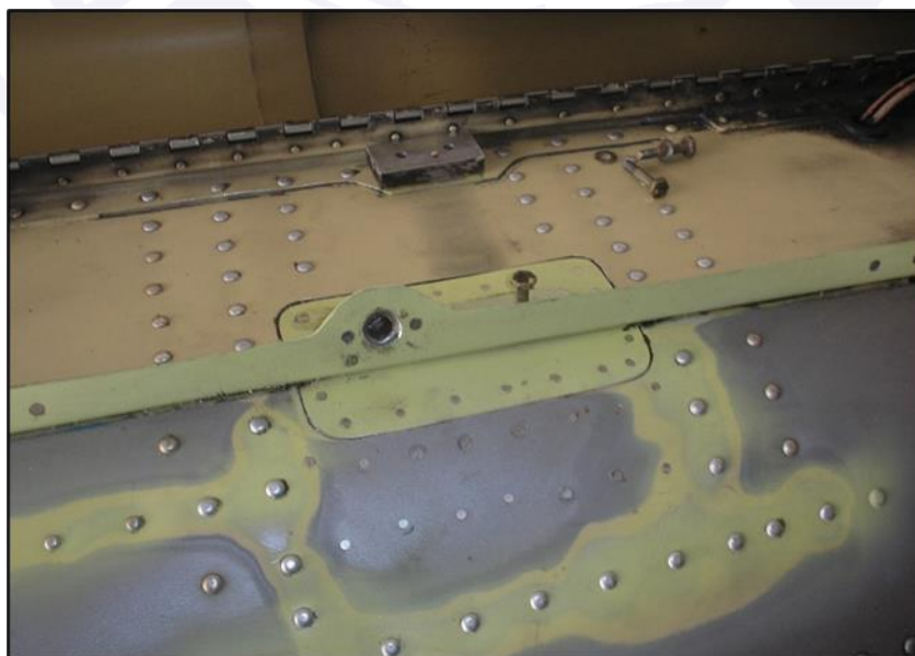
Figure 8 - Image of the external view of the redone repair.
