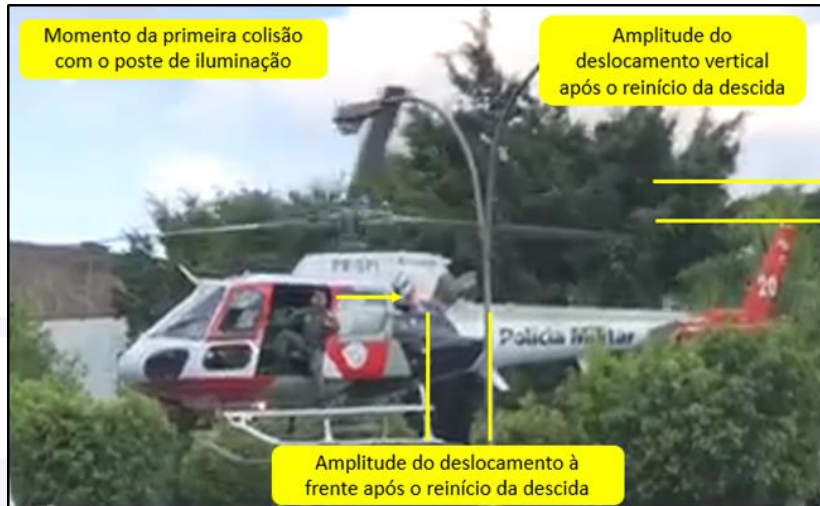
Figure 10 - Precise moment of the first collision of the main rotor against the lamppost. Source: Image captured from video provided by an observer of the accident.
