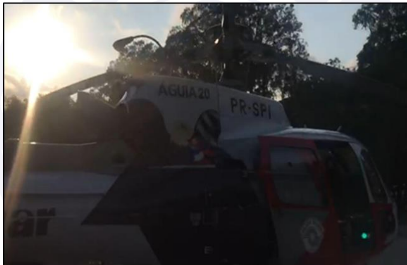
Figure 13 - Position of the sun relatively to the aircraft, immediately after the accident.
