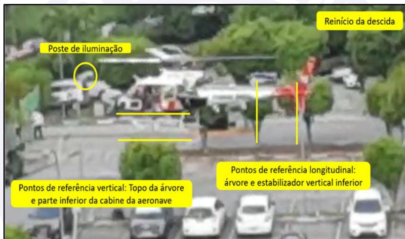
Figure 11 – Moment at which the PIC was performing a prolonged hover. Source: Image captured from a video provided by an observer of the accident located at the hospital.
