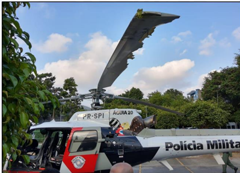
Figure 1 - View of the damage sustained by the PR-SPI at the accident site.
