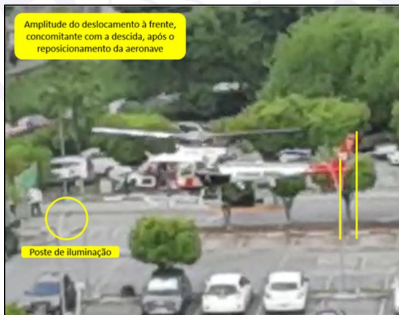
Figure 8 - Moment subsequent to the previous image, referencing the forward displacement in relation to the terrain. Source: Image captured from video provided by an observer of the accident.
