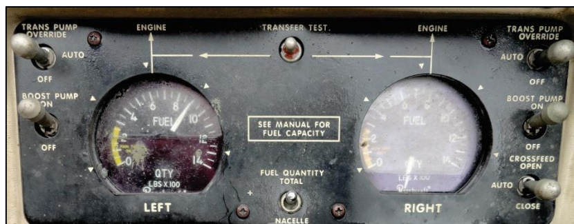
Figure 35 - Fuel control panel.
