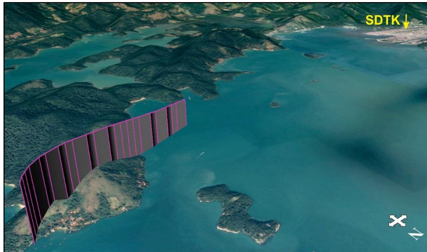
Figure 50 - Aircraft trajectory profile during the first approach attempt, according to aircraft EGPWS data.
