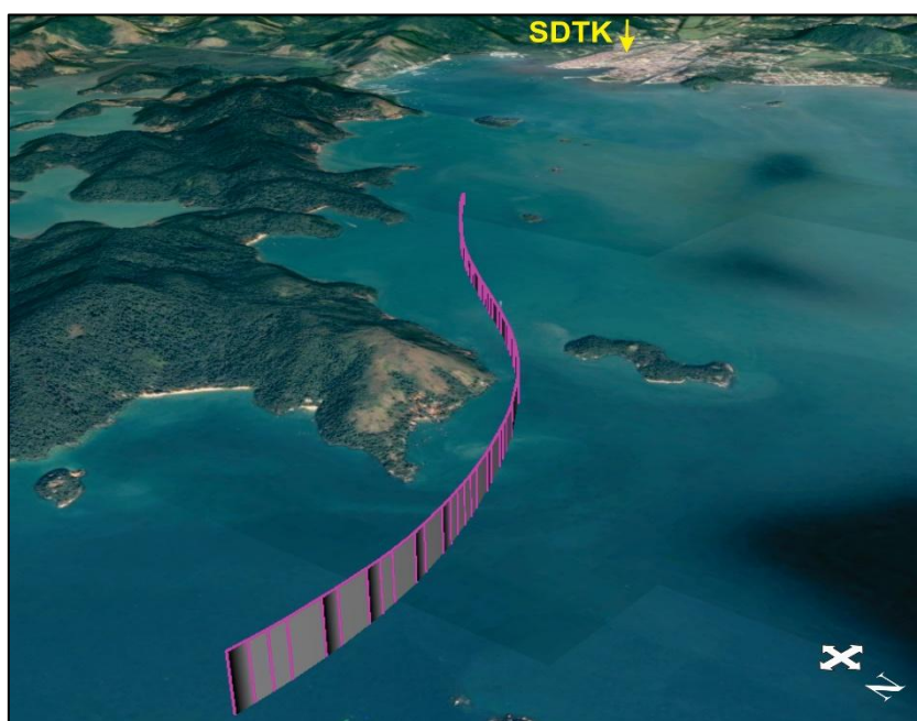
Figure 51 - Aircraft trajectory profile during the second approach attempt, according to the EGPWS data of the aircraft.
