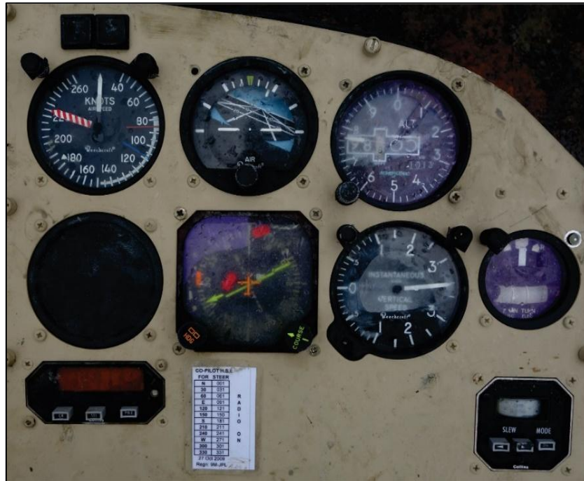
Figure 32 - Right-hand station instrument panel.
