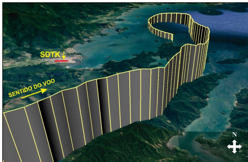
Figure 49 - Reconstruction of the descent profile of the aircraft, according to the RADAR air traffic control data.
