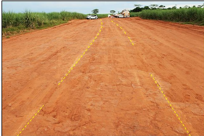
Figure 8 - Braking marks left by the aircraft in the moments before the collision with the vehicle, highlighted by dotted lines.
