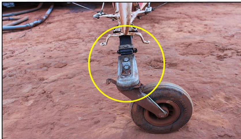
Figure 6 - Auxiliary landing gear, highlighting the absence of springs of the connection with the steering rudder.
