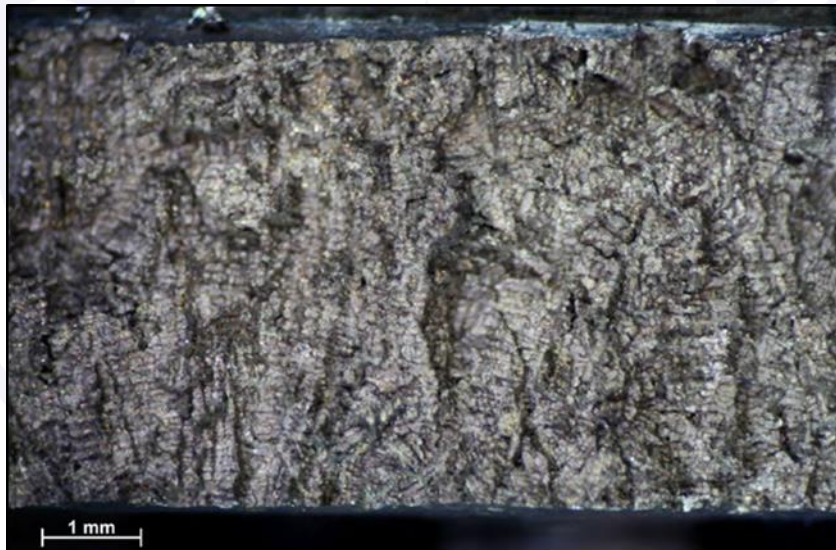
Figure 20 - Image showing the fracture region on a PT blade. Source: Investigation Report GEAC.
