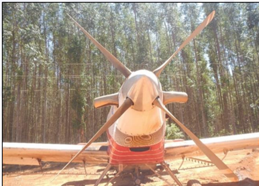
Figure 4 - Image of the aircraft propeller with the blades in the feathered position.
