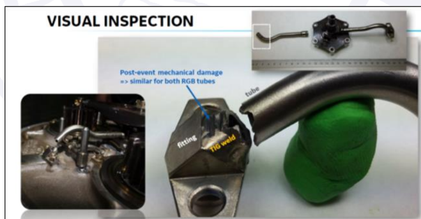
Figure 13 - Images of the fractured RGB Oil Tube obtained at the engine disassembly. Source: Investigation Report GEAC.
