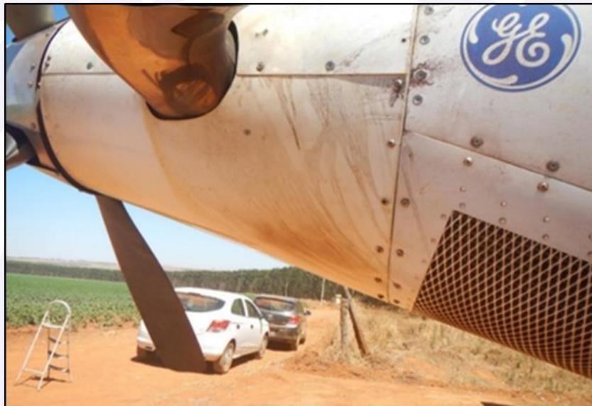
Figure 5 - Oil marks on the engine cowling.
