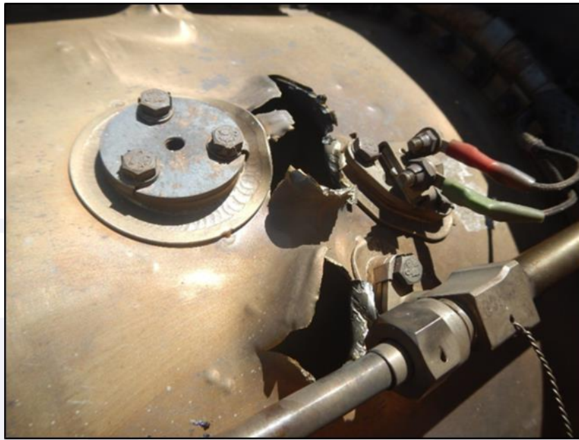
Figure 9 - Evidence of severe internal damage to the engine.
