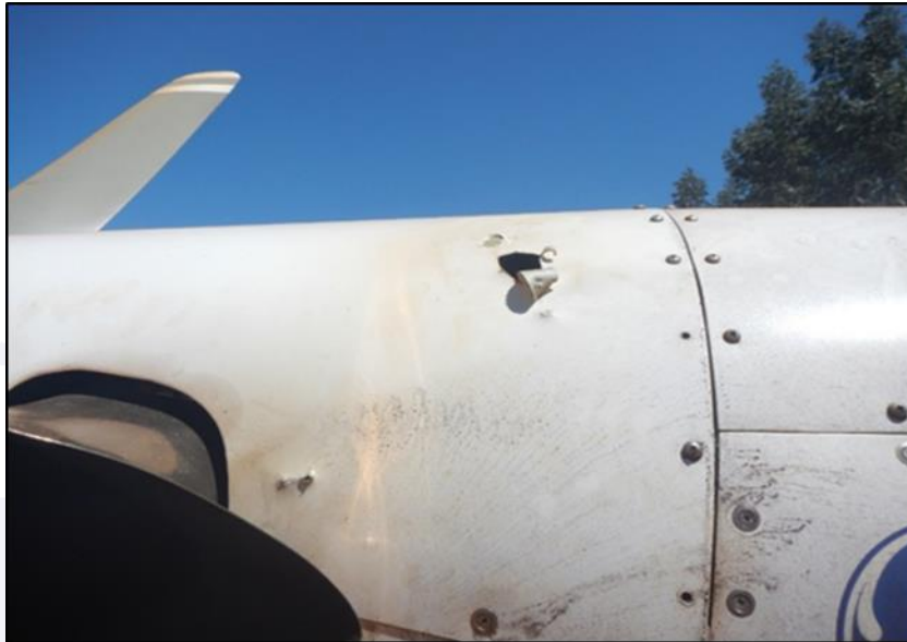
Figure 6 - Damage with perforation on the left side of the engine cowling.
