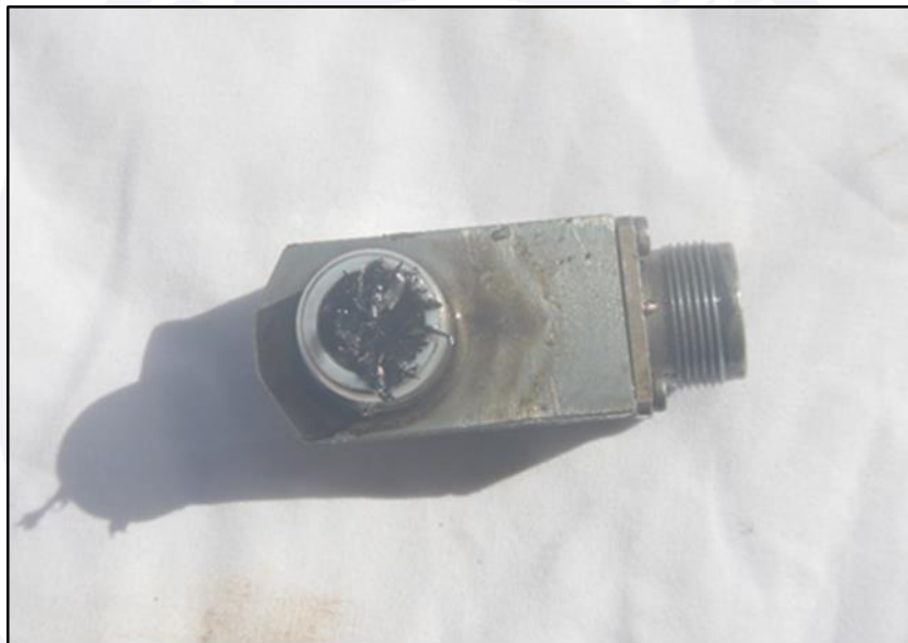
Figure 10 - Magnetic plug of the engine filing detection system contaminated with metal particles.
