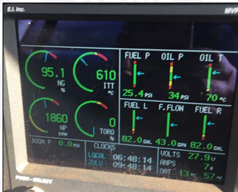
Figure 27 - Image recorded by the PIC showing the torque indication on the MVP-50T screen.
