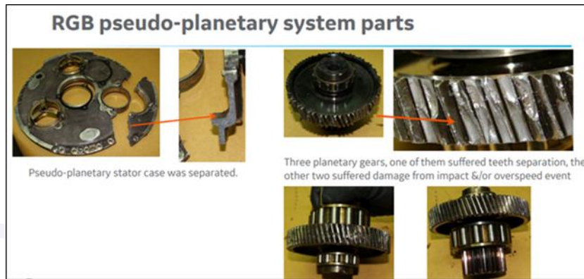
Figure 16 - Damaged planetary gears. Source: Investigation Report GEAC.
