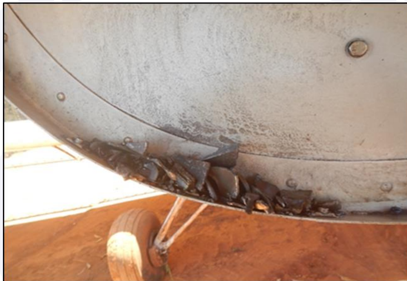
Figure 7 - Debris found inside the engine compartment.
