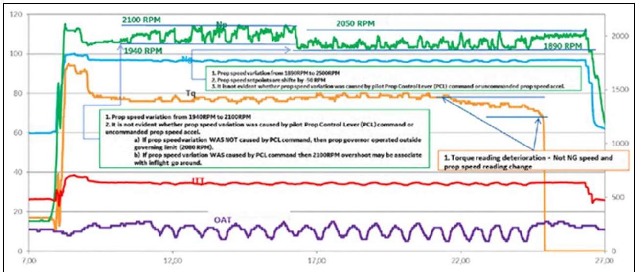
Figure 26 - Diagram of aircraft engine parameters in the first complete flight. Source: Investigation Report GEAC.
