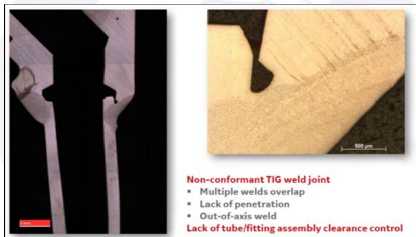
Figure 15 - Image obtained during the metallographic examination of the sectioned tube, highlighting welding characteristics different from those required.
