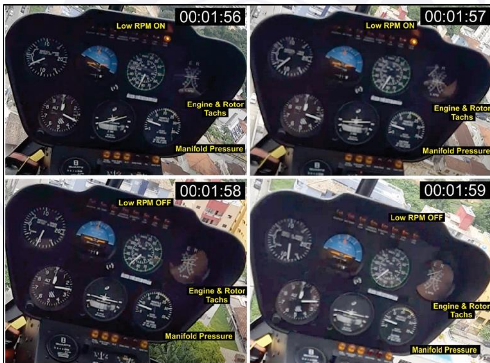
Figure 19 - Variation in engine RPM, while the rotor remains constant at 80%, and low RPM light "cycling".
