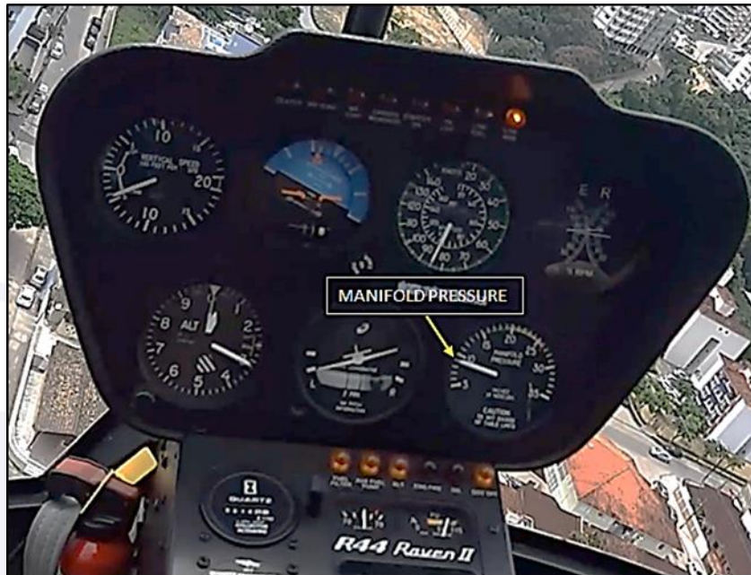
Figure 24 - Indication of the intake pressure of the PR-RMZ engine.
