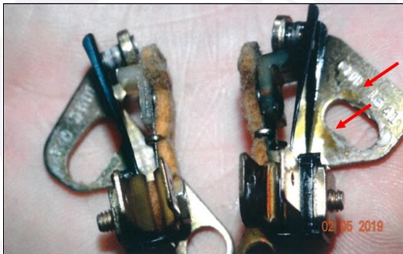
Figure 8 - Lubricating oil residue on the contact breaker of the right-hand magneto.
