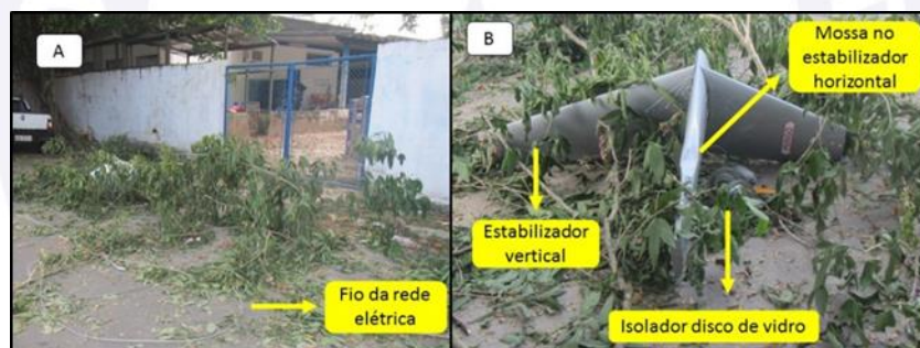
Figure 7 - Electrical network wire (A) / Aircraft vertical and horizontal stabilizers and insulator (B).
