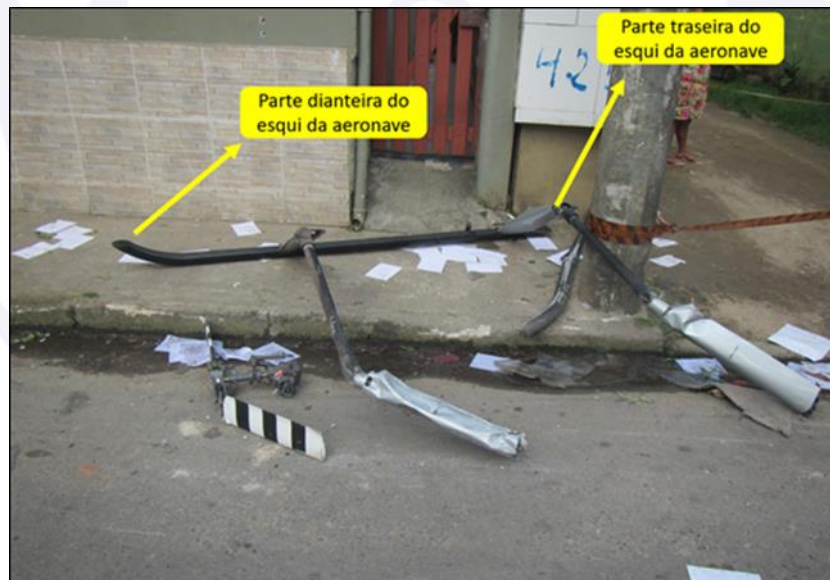
Figure 5 - Helicopter skid after collision against a public utility-pole.
