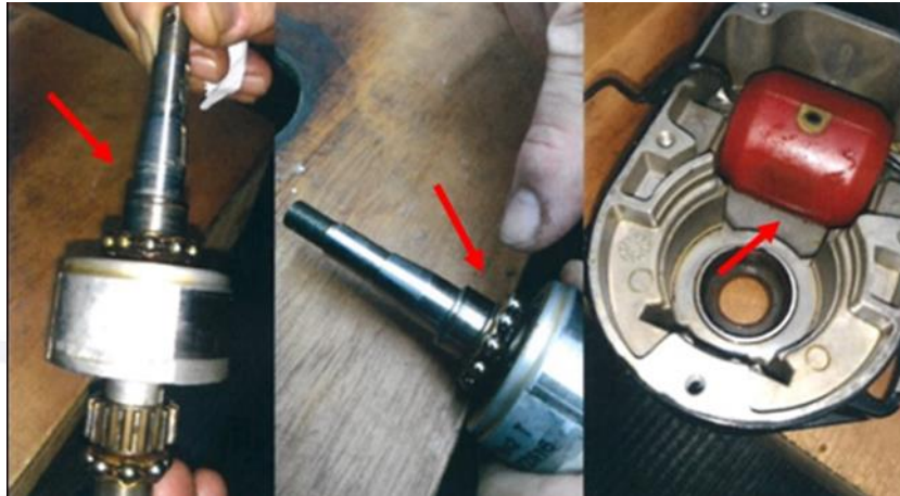
Figure 10 - Presence of lubricating oil in the rotor and right-hand magneto housing.
