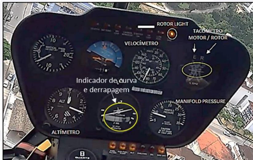
Figure 17 - Image captured by the passenger's camera, moments after activation of the low rotor rotation alarm.
