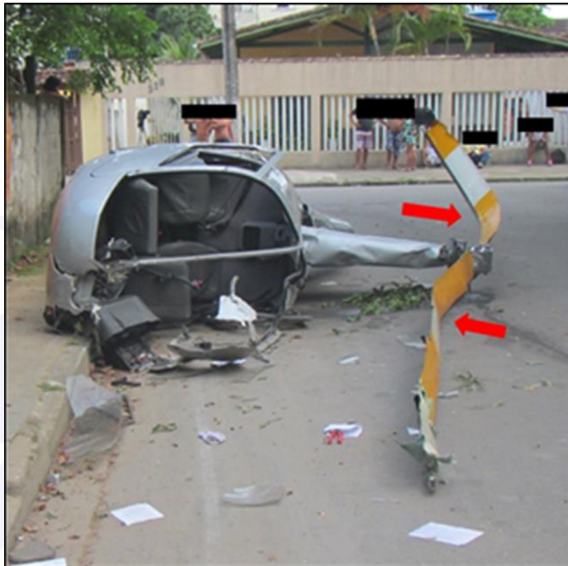
Figure 6 - The red arrows show the main rotor blades bent upwards. One of the blades rotated 180° in the longitudinal axis and became inverted (upside down) in relation to the other one.
