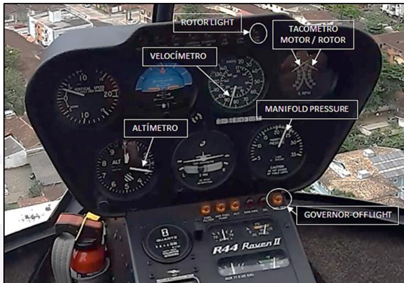
Figure 16 - PR-RMZ panel, without discrepancies, during the climb after takeoff.
