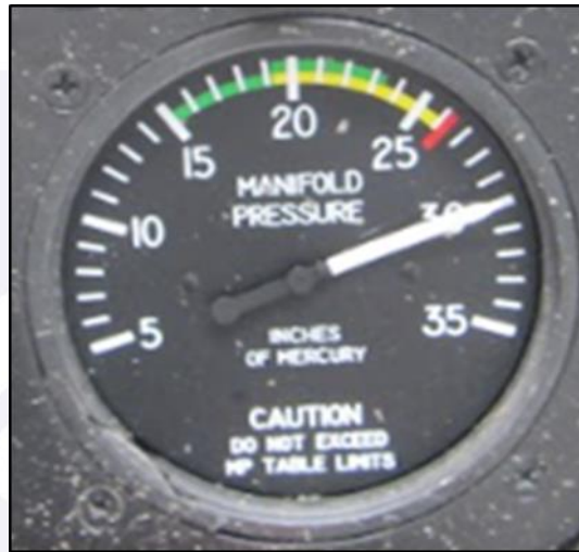
Figure 2 - PR-RMZ engine intake pressure indicator, after the accident.
