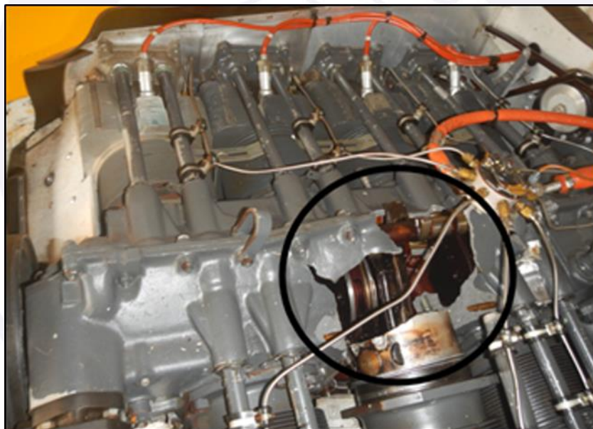
Figure 4 - Upper view of the engine showing the rupture of cylinder No. 4.
