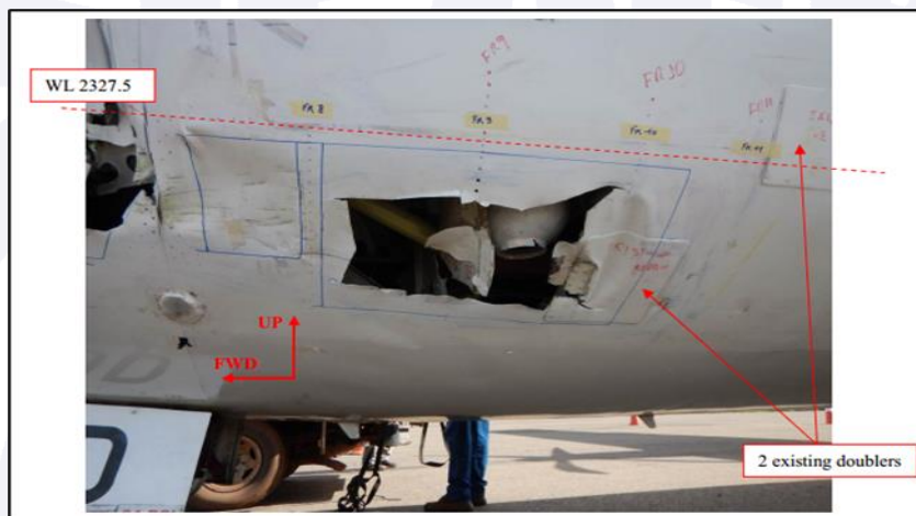
Figure 5 - Perforations in the left front Skin Panel (Source: ATR).
