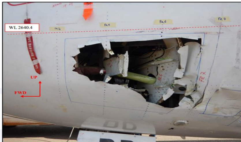
Figure 4 - Perforations in the left front Skin Panel (Source: ATR).
