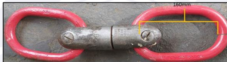
Figure 2 - Rings identical to those used to hook the external load at the time of the occurrence. The yellow lines indicate the inside measurement of the ring.
