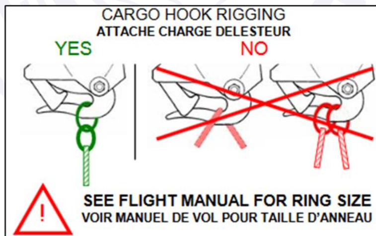
Figure 3 - Plate containing loading guidelines for the cargo hook. Source: ASB nº 04A004, from 12MAY2009.
