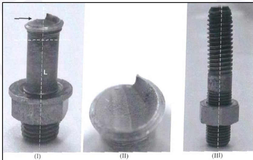
Figure 7 - Image of the right-hand engine crankcase thru bolts extracted from the analysis report.
