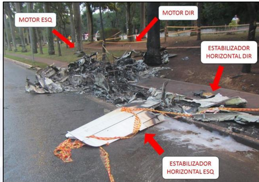
Figure 4 – Aircraft wreckage in the crash site.
