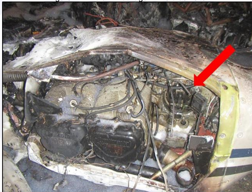
Figure 5 – Detail of the right-hand engine without the cylinder no. 5.
