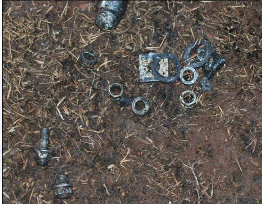
Figure 6 – Image of the crankcase through-bolts of the right-hand engine.
