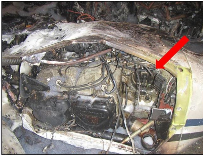
Figure 5 – Detail of the right-hand engine without the cylinder number 5.
