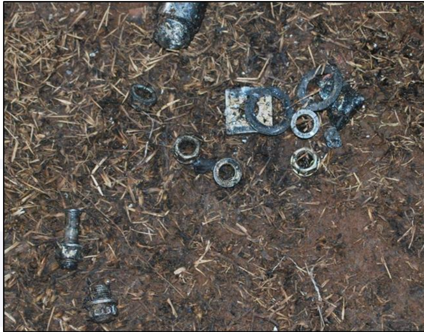
Figure 6 – Image of fragments of studs and nuts of the right engine.
