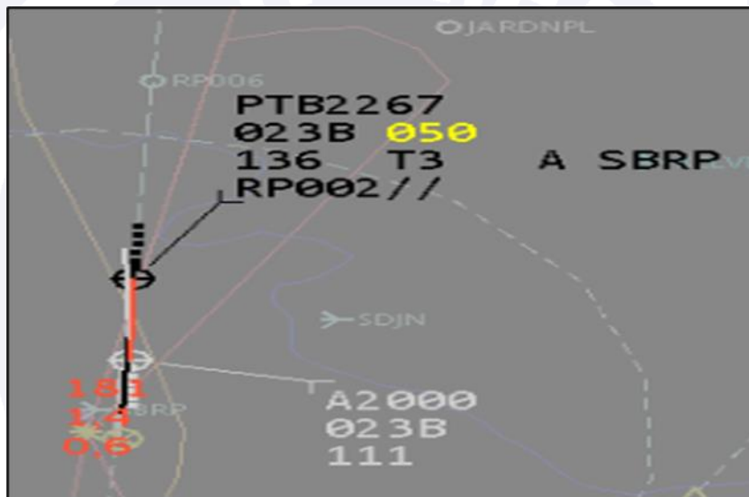
Figure 8 - RADAR image showing the aircraft on the same axis and at the same level.
