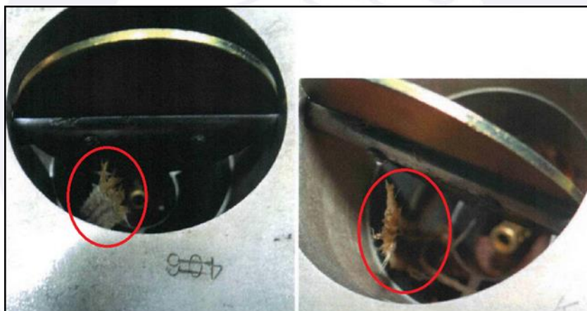
Figure 6 – Images of the foreign material lodged in the carburetor venturi.
