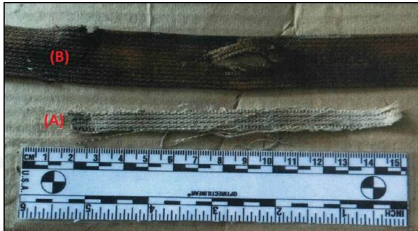
Figure 7 – (A) Fabric found inside the carburetor – (B) Fabric from the aircraft fuselage.
