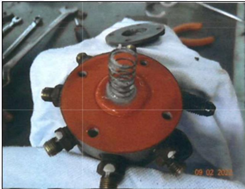
Figure 7 - View of the fuel distributor diaphragm with salt water and corrosion on its spring.
