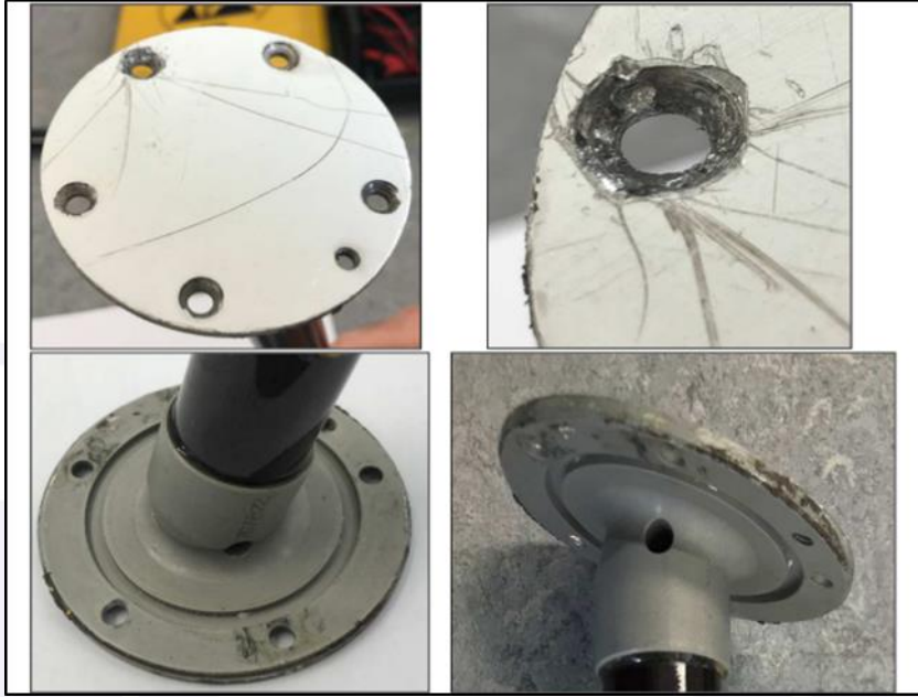
Figure 15 - Damage to the P/N 768-100 S/N 516 7 fuel-probe head. Source: SAFRAN Investigation Report.
