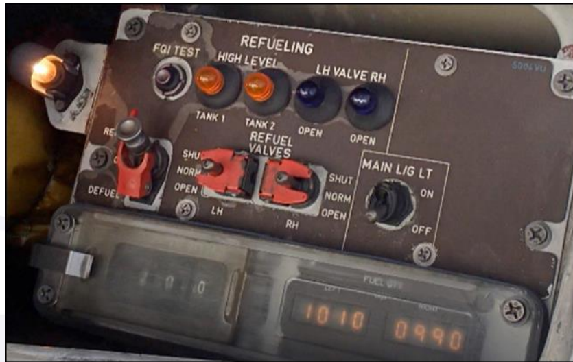
Figure 25 - ATR-72 Refuel Control Panel (illustrative image). Source: ATR Systems - Fuel System.
