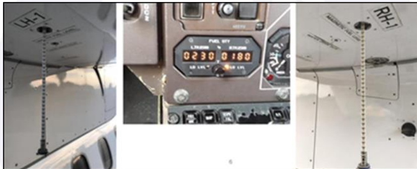
Figure 9 - Indication of the PR-MPY FQI and Fuel-Level Magnetic Indicators measured after the landing in SBIH.
