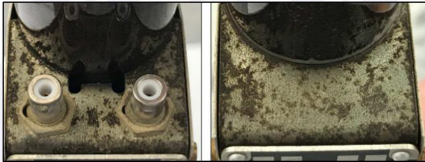
Figure 16 - Oxidation in the electrical box of the P/N 768-100 S/N 516 7 fuel probe. Source: SAFRAN Investigation Report.
