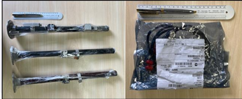
Figure 10 - Fuel probes and number-3 probe wiring sent for testing.
