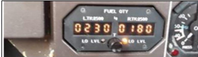
Figure 23 - PR-MPY LO LVL Fuel of Engine no. 2 illuminated in SBIH.
