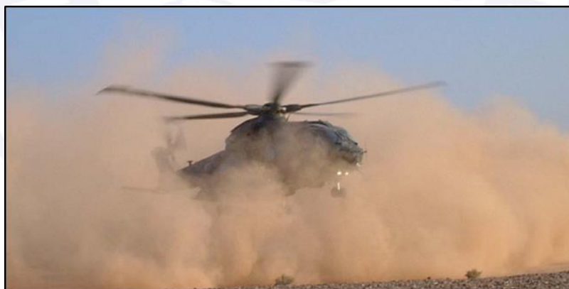
Figure 23 - Helicopter entering a brownout condition. Source: Technical Report - Rotary-Wing Brownout Mitigation: Technologies and Training .
