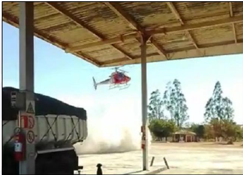
Figure 40 – Rise of particles in the landing area caused by the downwash of the main rotor.
