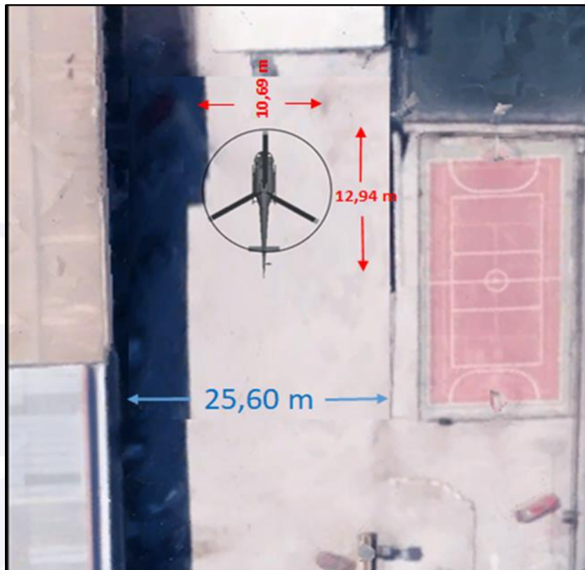
Figure 21 - Croquis of the accident site with the dimensions of the landing area and of the helicopter. Source: adapted from Google Maps .
