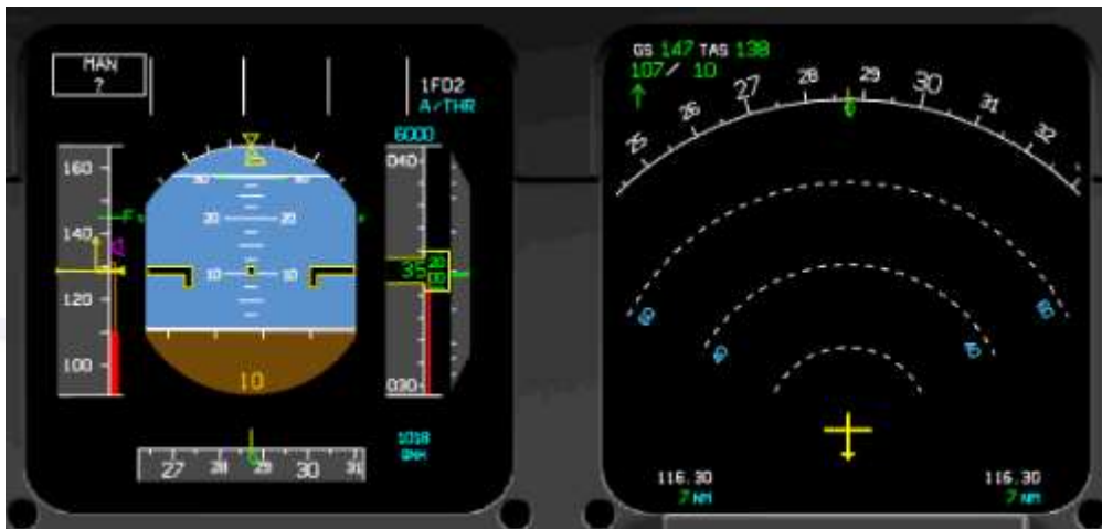
Figure 20 - FDM data on PFD and ND shortly after the aircraft becomes airborne, during the go-around procedure.
