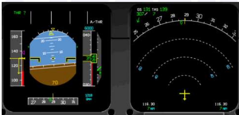
Figure 18 - FDM data on PFD and ND showing the beginning of the go-around procedure, the moment the levers were pushed forward, passing through the FLX-MCT thrust position, hitting TOGA thrust position, 1 second later.
