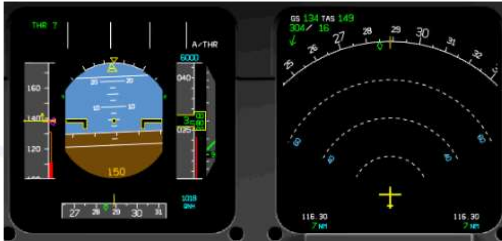
Figure 17 - FDM data on PFD and ND.
