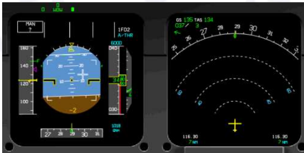
Figure 19 - FDM data on PFD and ND at the moment the right main landing gear touches the ground.
