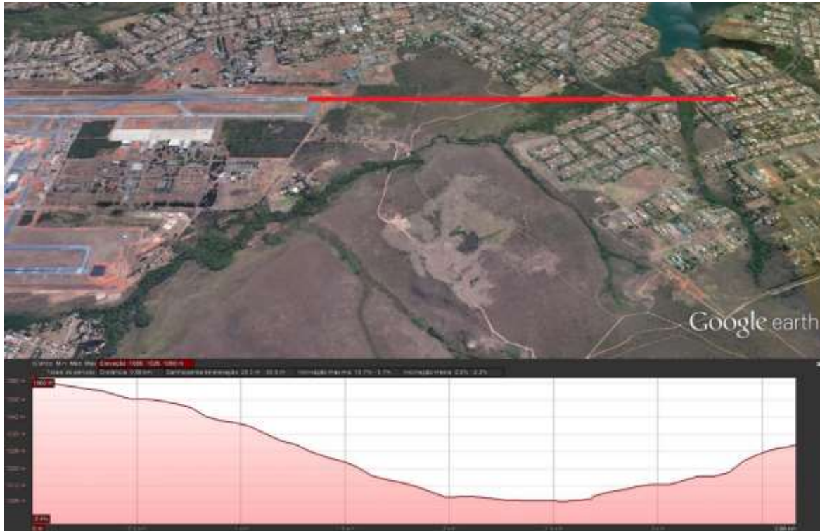
Figure 13 – Vertical section along the red line, prior to the RWY 29R of SBRR. Credit: Google Earth.
