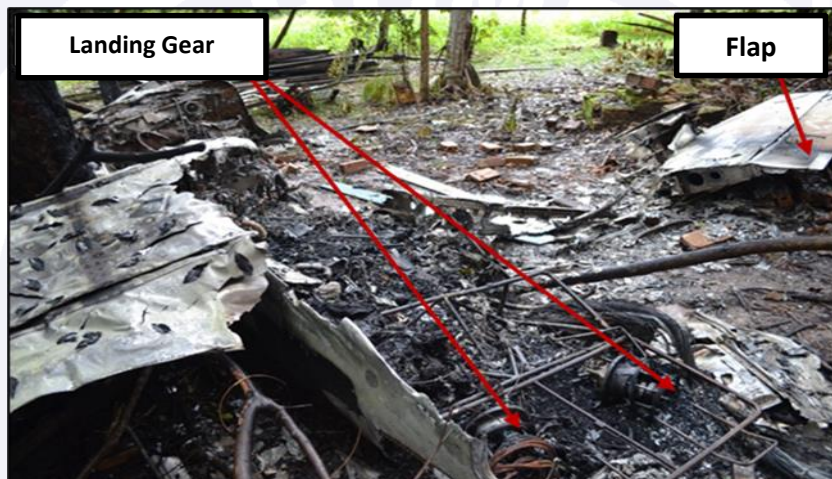
Figure 4 - Aircraft destroyed by fire. Landing gear and flaps retracted.
