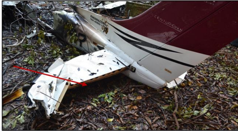
Figure 3 - Left horizontal stabilizer without elevator.
