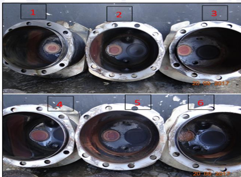
Figure 5 - Interior of the cylinders. Exhaust valves with reddish coloration.
