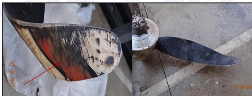
Figure 13 - Scratches and dents on the propeller blades.
