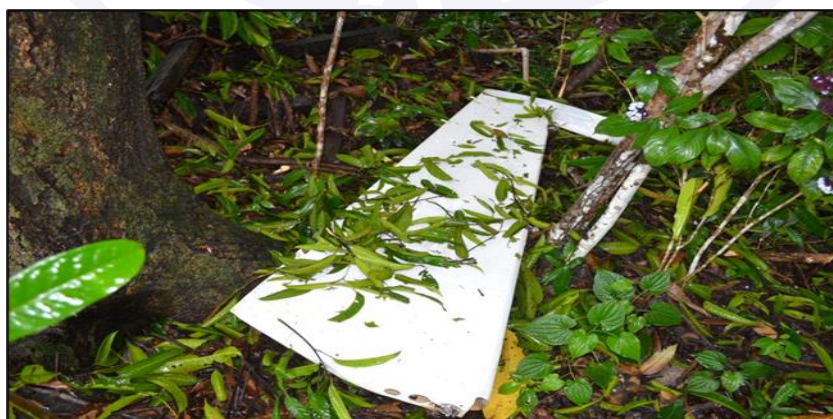
Figure 2 - Left elevator found near the site of the first impact.
