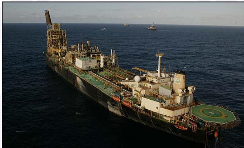
Figure 14 - View of the P-35 platform ship, highlighting the helideck at the stern of the ship.
