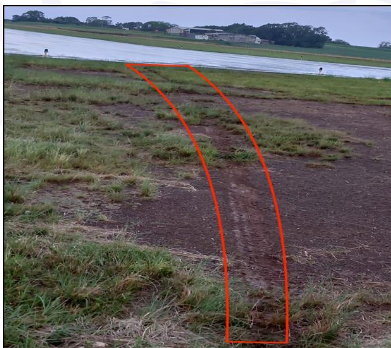
Figure 7 - Aircraft trajectory after runway excursion past the departure end of SSIJ RWY 36.
