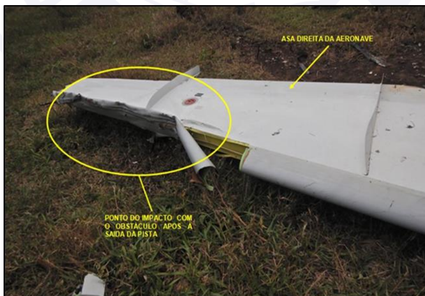
Figure 8 – Right-hand wing of the aircraft showing damage resulting from the impact with the obstacle after exiting the runway.
