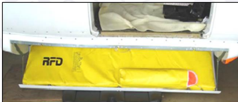
Figure 5 - S-76C++ helicopter's life raft compartment.
