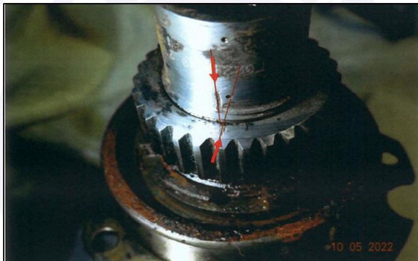
Figure 30 - View of the misalignment of the marks between the input pinion of the module 05 of the SN 42326TEC engine and the shaft.
