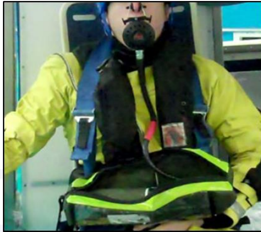
Compressed Air Emergency Breathing System (CA EBS).
