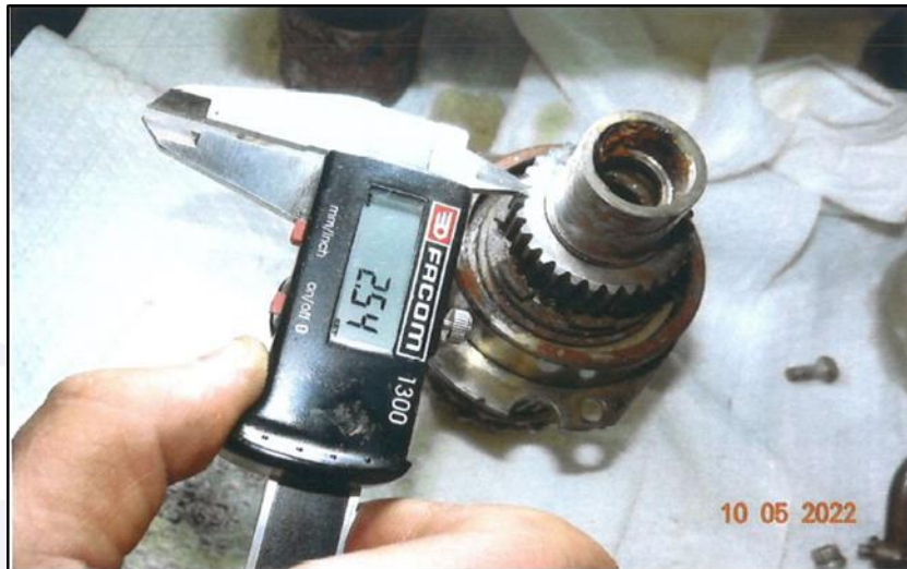
Figure 31 - Measurement of the 2.54 mm misalignment observed between marks.
