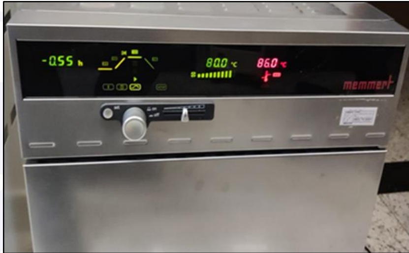
Figure 19 - Oven for drying the memory board, in operation at the LABDATA.
