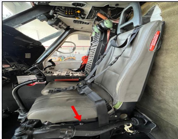
Figure 7 - View of the S-76C++ helicopter's inertia reel control lever of the left-hand pilot's seat.
