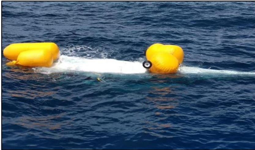
Figure 22 - View of the PR-LCT after the crash, showing the four inflated emergency floats, which kept the helicopter afloat just below the sea surface.
