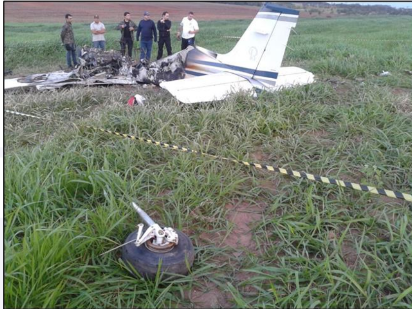
Figure 5 - Broken right main landing gear.
