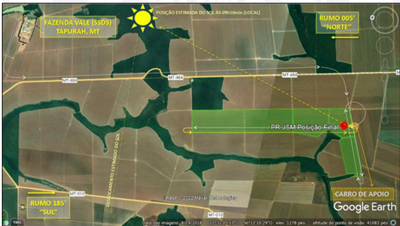
Figure 3 - Sketch of the trajectory flown by the aircraft.
