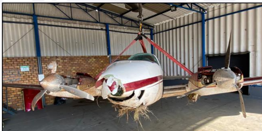
Figure 5 - View of the damage sustained by the propeller blades and fuselage.
