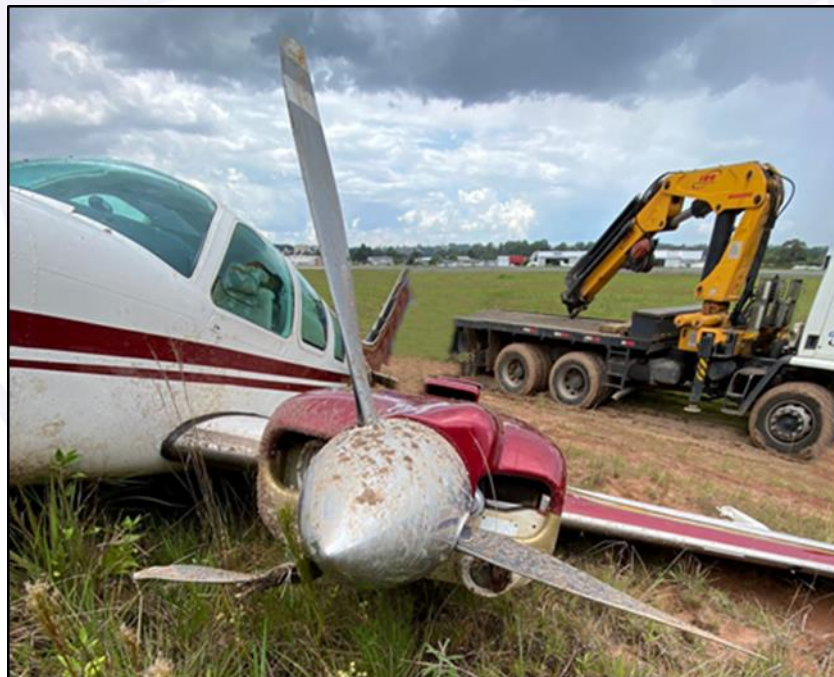
Figure 3 - Left engine's propeller blades in the feathered position showing longitudinal damage to one of the blades.
