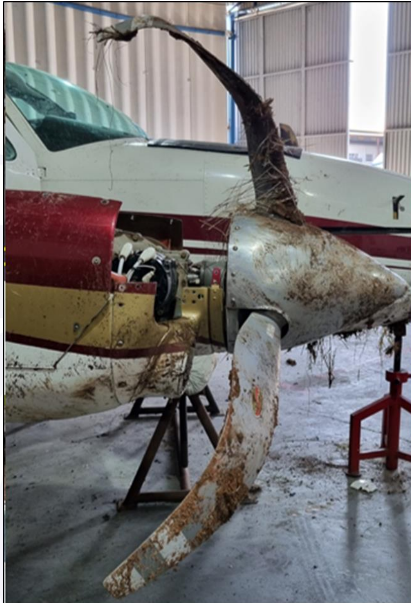
Figure 4 - Right engine propeller blades not feathered, exhibiting longitudinal damage.
