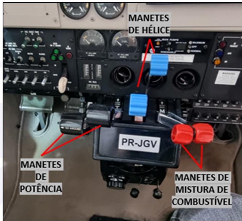
Figure 6 - Image of the throttle, propeller, and fuel lever positions after the accident.
