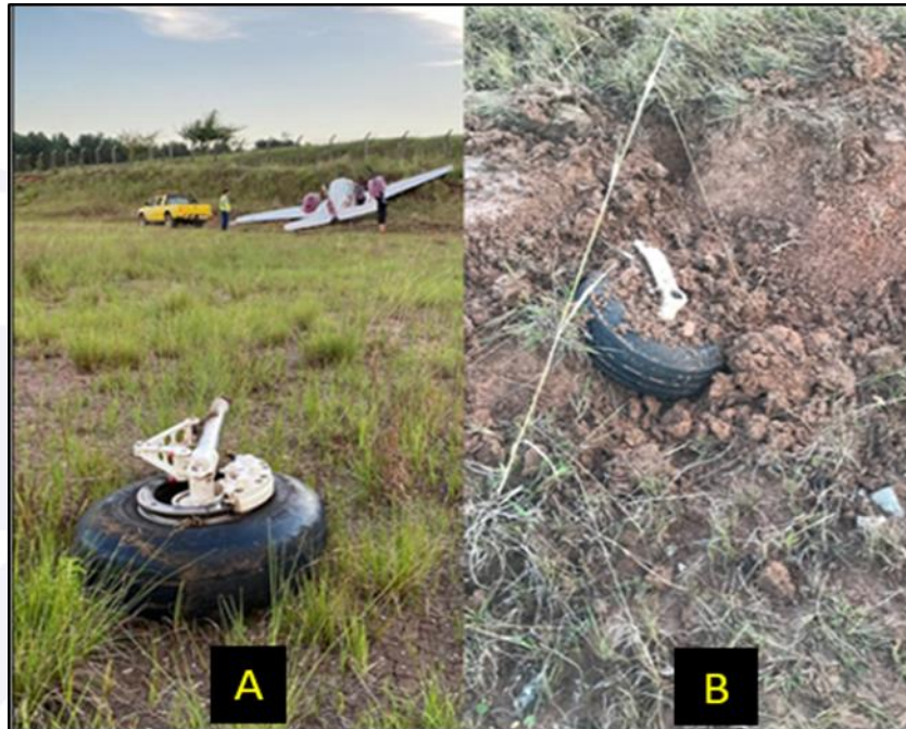
Figure 2 - Left main landing gear (A) and nose landing gear (B).
