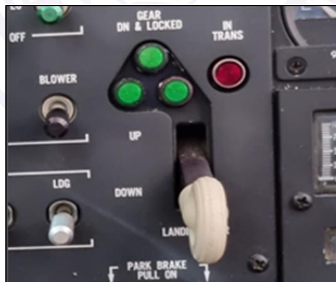
Figure 14 - Landing gear lever in the DOWN position.
