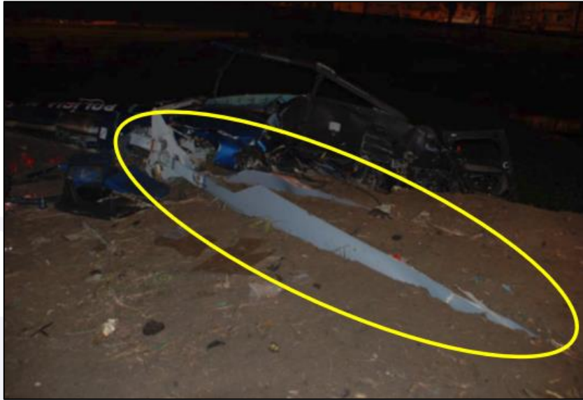
Figure 3 – Wreckage seen from above, highlighting two of the main rotor blades partially buried in the terrain.
