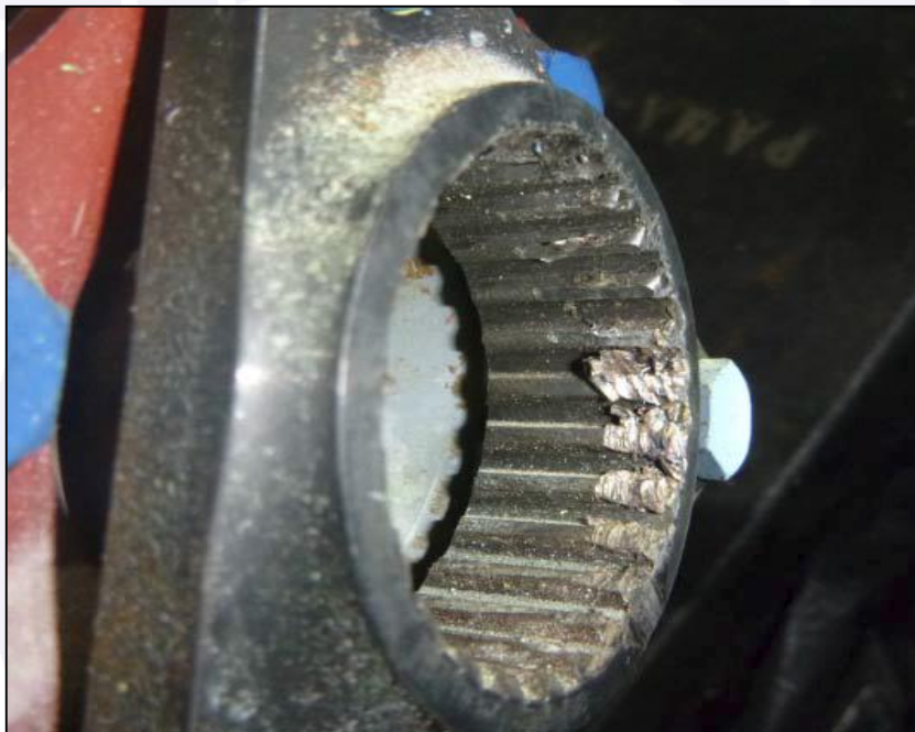
Figure 9 - Evidence of rotational damage on the inner splines of the engine shaft flange.
