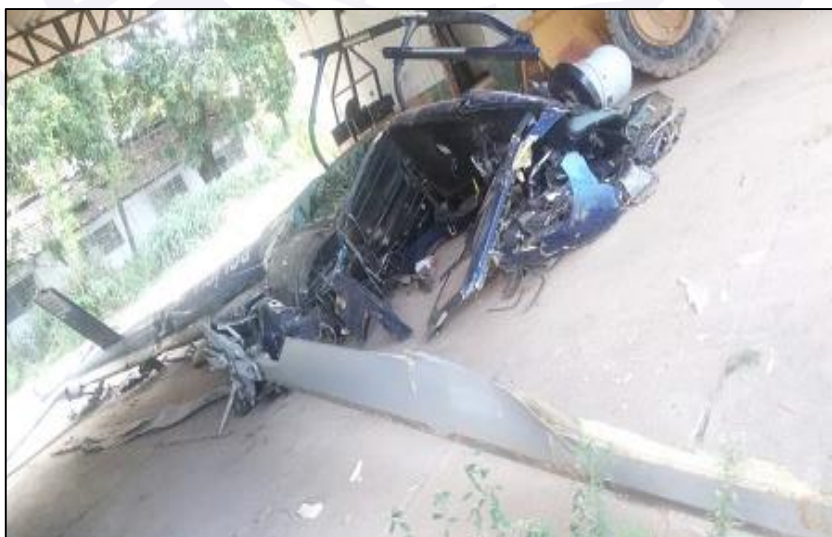
Figure 8 – Greater damage to the right side of the aircraft with characteristics of flattening.
