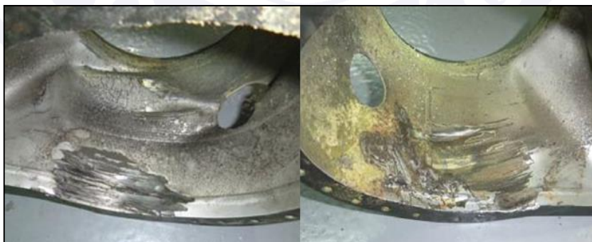
Figure 10 - Evidence of rotational damage between the engine connection tube and the engine output shaft (freewheel assembly).
