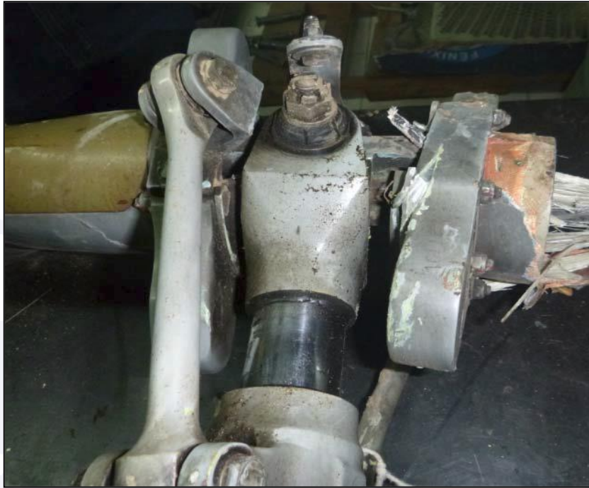
Figure 14 – Tail rotor head: damage compatible with aircraft impact with the ground.
