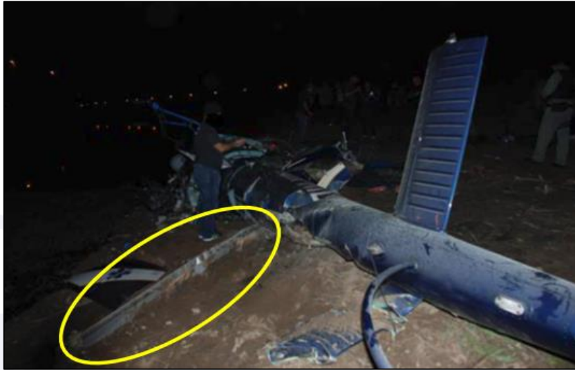
Figure 6 – Rear of the aircraft (left side) with the third blade of the main rotor in highlight.
