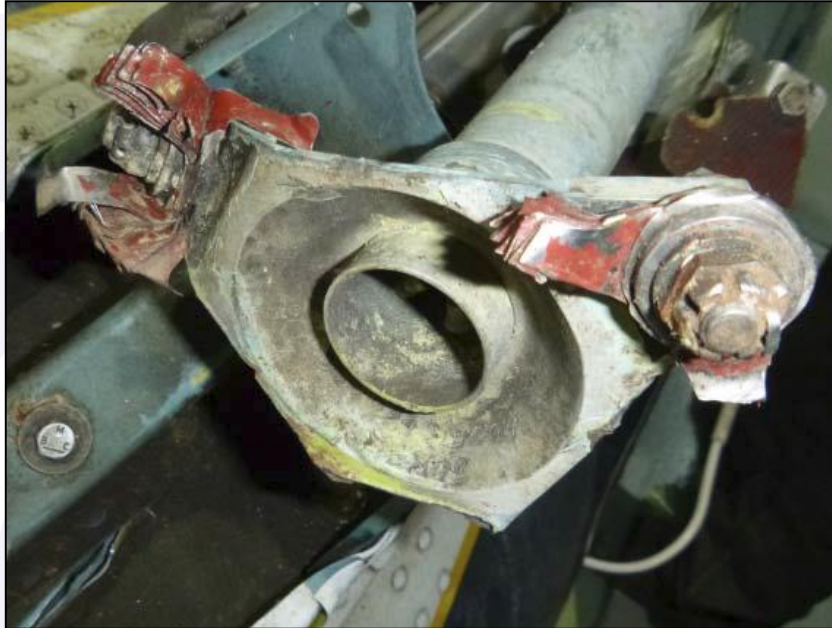
Figure 12 – Evidence of overload-induced damage to the remaining parts of the flexible coupling of the tail-rotor drive shaft.
