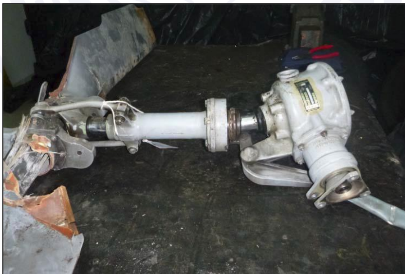
Figure 13 – Tail rotor gear box: damage compatible with impact of the aircraft with the ground.
