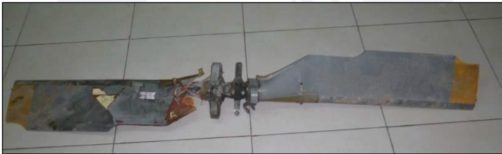
Figure 15 – Tail rotor blades: damage compatible with impact of the aircraft with the ground.
