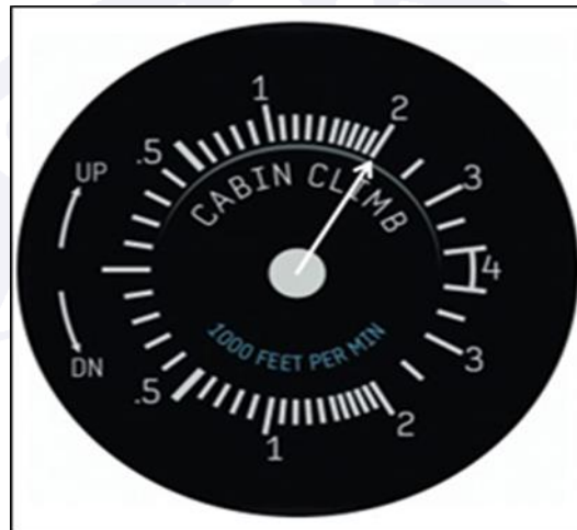
Figure 9 - Representation of a cabin climb marking 2,000ft/min positive. Source: Adapted from FCOM.
