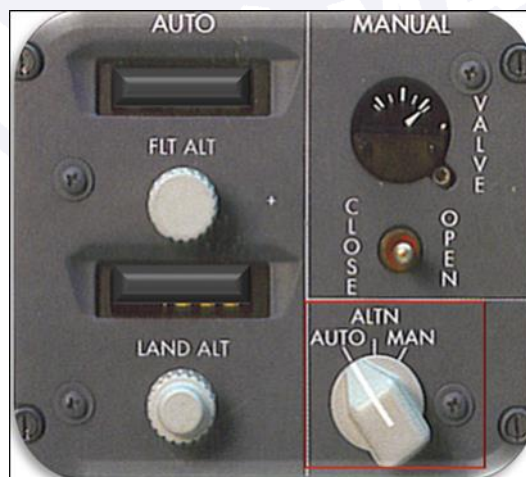
Figure 10 - Pressurization control modes.
