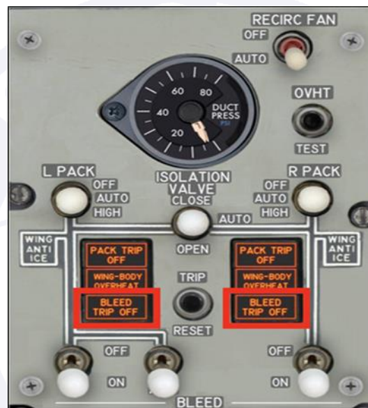
Figure 7 - Pressurization panel, with emphasis on the BLEED TRIP OFF lights. Source: FCOM.
