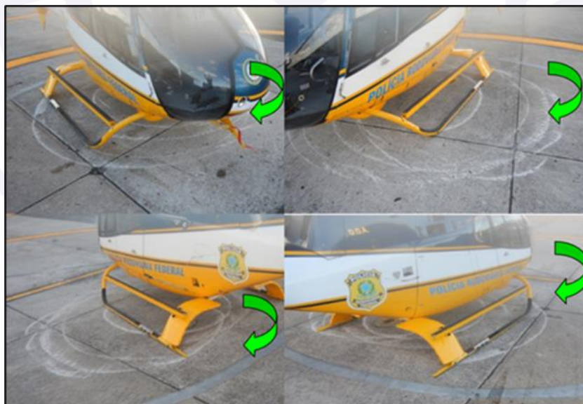
Figure 6- Details of the markings on the ground after the ground turn (the green arrow indicates the direction of rotation of the aircraft).
