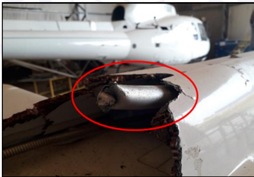
Figure 9 – Tail rotor drive shaft with torsional failure.
