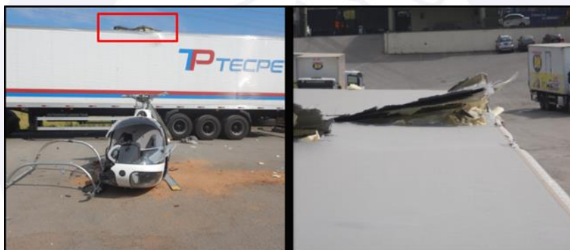
Figure 3 – On the left, the point of impact on the truck; on the right, detail of the damage.
