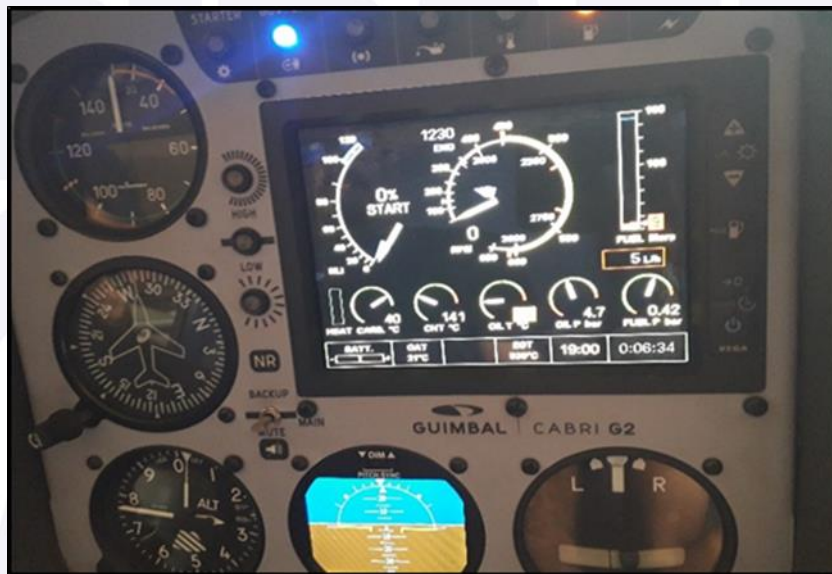
Figure 8 – Image of the instrument panel during engine run-up.
