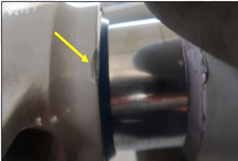
Figure 8 - Mark observed on the rotating control plate, caused by the contact of the tail rotor blade counterweight.
