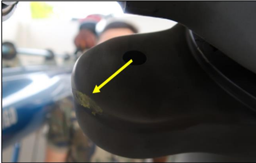
Figure 7 - Approximate view of the mark left on the counterweight, due to contact with the rotating control plate.
