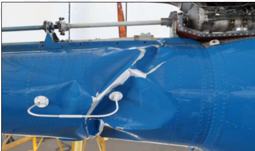
Figure 1 - Damage to the aircraft tail cone (seen from the right side).
