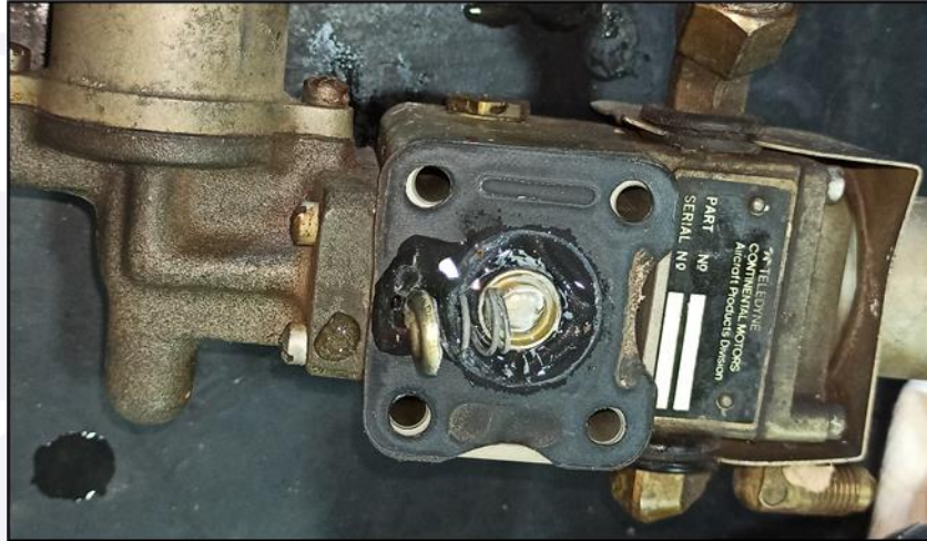
Figure 6 - View of the disassembly of the mechanical fuel pump.
