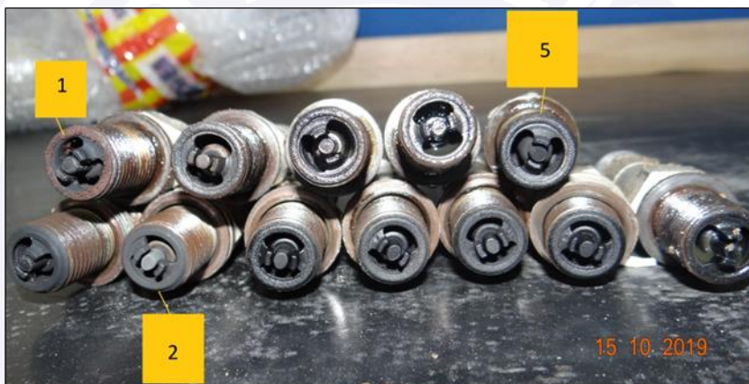
Figure 9 - General view of the engine spark plugs. On the spark plugs of cylinders 1, 2 and 5, the presence of black soot was evident.
