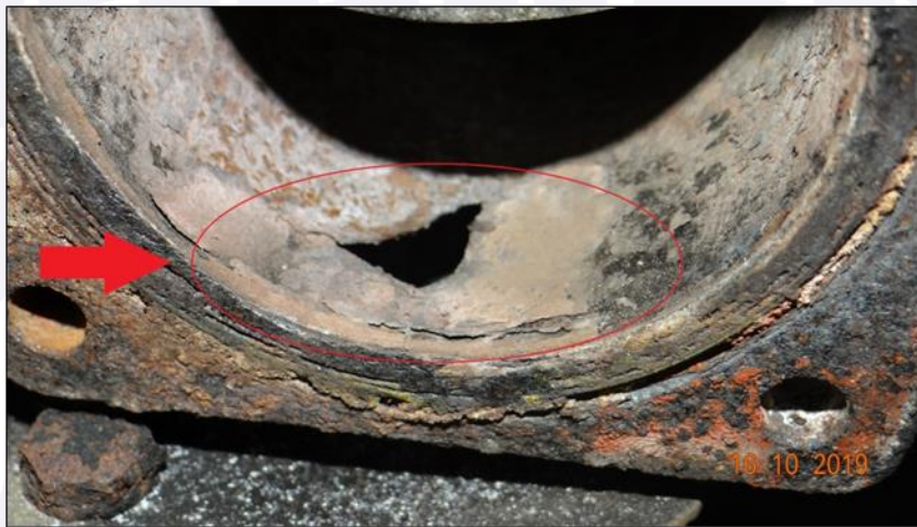
Figure 15 - View of the crack and hole observed inside the throttle body, caused by severe corrosion.
