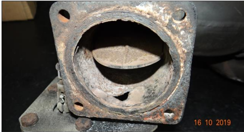
Figure 14 - View of severe corrosion on the inside of the throttle body.
