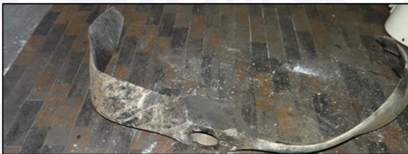
Figure 4 - General view of the propeller with the blade tips facing backwards.
