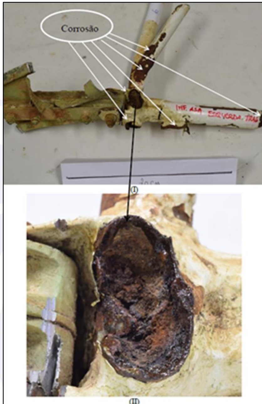
Figure 9 – View of the lower truss of the left wing showing widespread corrosion.
