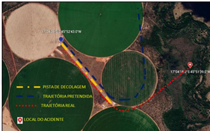
Figure 10 – Sketch of the aircraft's trajectory. The dashed blue line shows the usual profile. The dotted red line shows an estimate of the trajectory during this accident.
