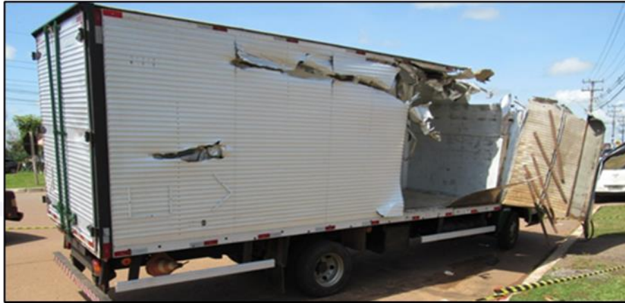
Figure 2 - Condition of the truck after the impact against the main rotor of the aircraft.
