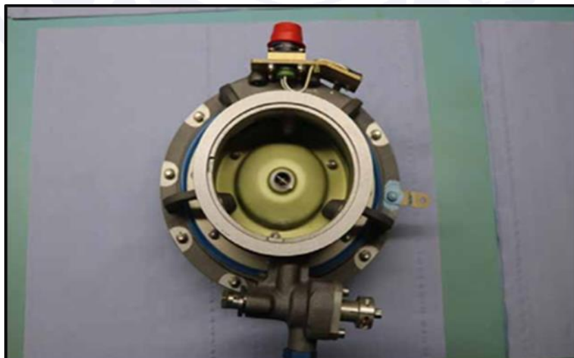
Figure 8 - Positive Relief Valve viewed towards the external, non-pressurized section of the aircraft.
