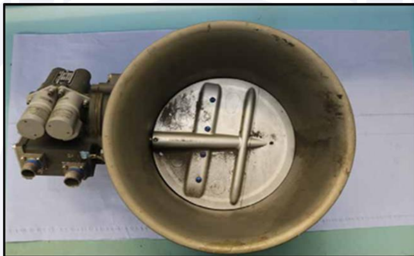
Figure 7 - Outflow Valve overview.
