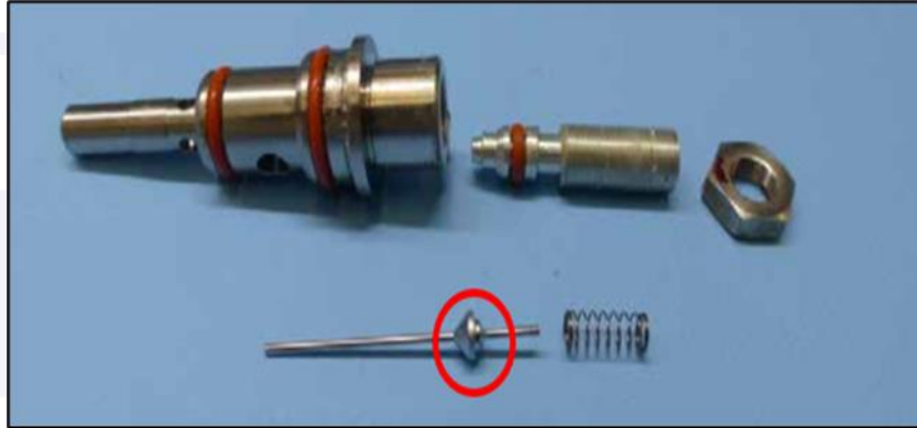
Figure 13 - Disassembly of the Needle of the Controller Unit. Highlighted, where signs of contamination were found.
