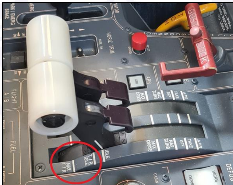
Figure 4 - T/R actuation range of the PR-AUR aircraft.
