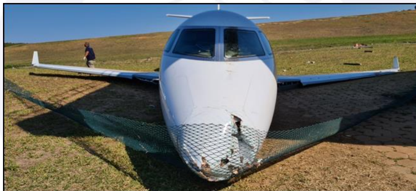
Figure 6 - Detail of the fence against which the aircraft collided after departing the runway.
