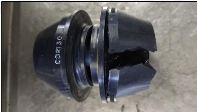
Figure 9 - Cracked rubber of one of the engine support shock absorbers.
