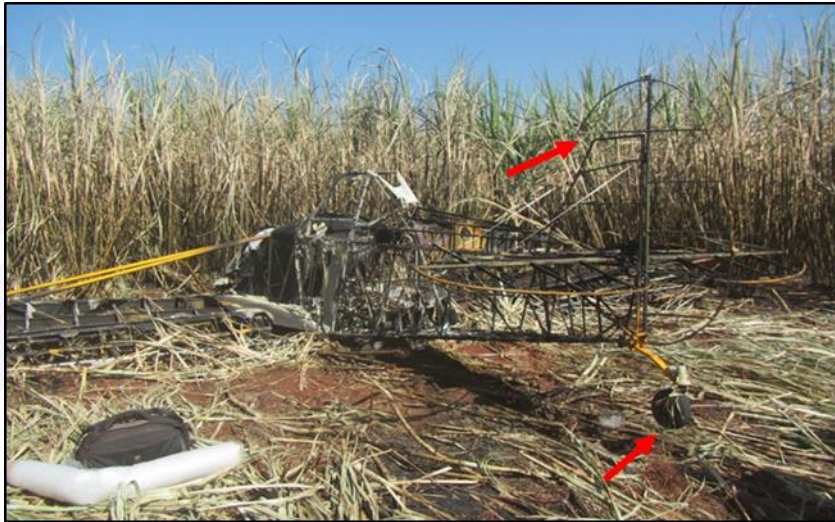
Figure 5 - Rudder deflected to the right, and tail-wheel of the aircraft.
