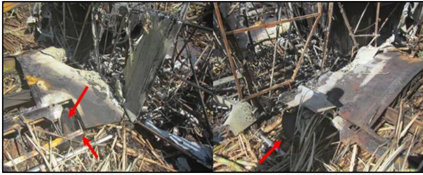
Figure 4 - Flap lowered, with the left- and right- main gear attached to the aircraft.
