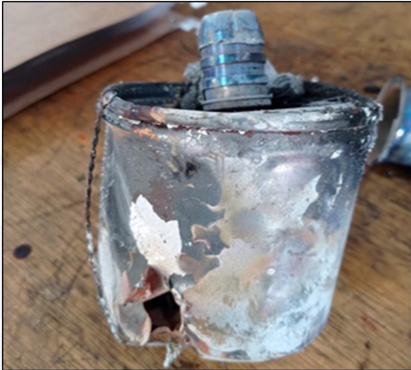
Figure 9 - Charred oil filter.
