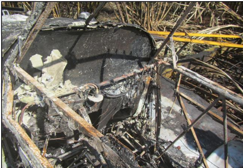
Figure 6 - Charred cabin and instrument panel.
