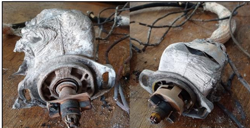
Figure 8 - View of the damaged engine magnetos.
