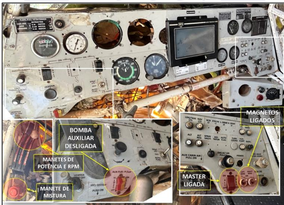
Figure 4 - Detail of the aircraft panel after the accident.
