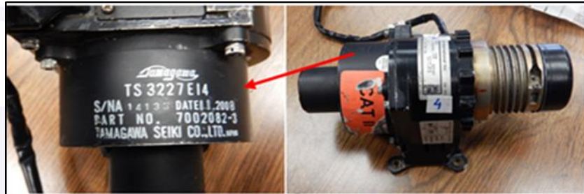
Figure 17 - Servo Drive and the identification of the electric engine.
