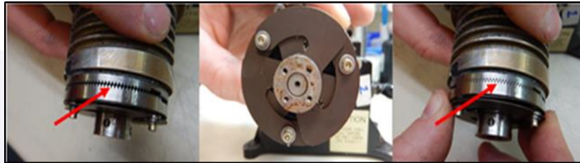
Figure 21 - Clutch disengaged, front view and manually engaged.
