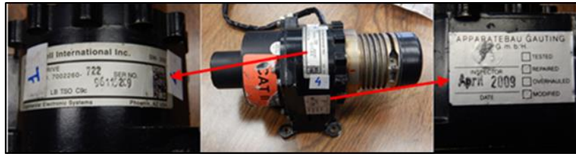
Figure 16 - Servo Drive and its identification plates.
