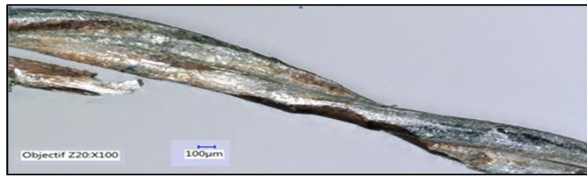
Figure 13 - Enlarged view of control cable wires removed from the Servo Drive with marks of plastic deformation and oxidation on the surface.
