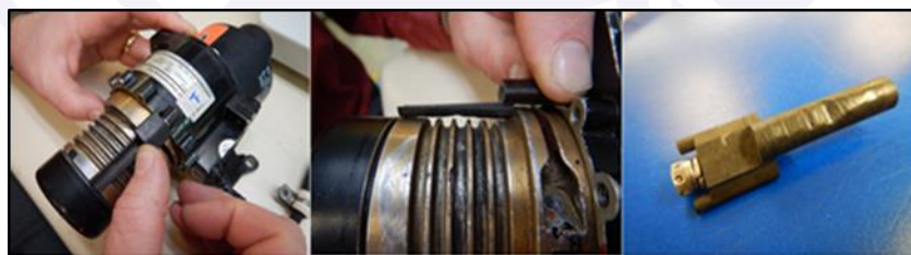
Figure 19 - Cable keeper positioned and a wear detail.
