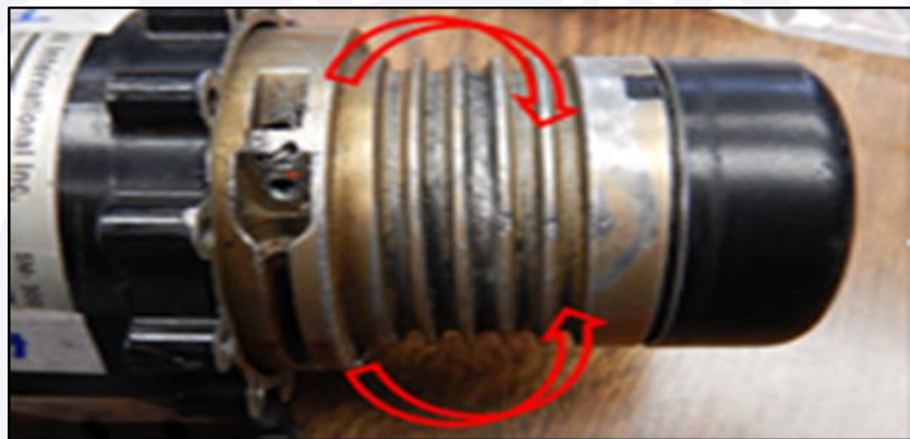
Figure 18 - Capstan free to rotate in both directions, clockwise and counterclockwise.
