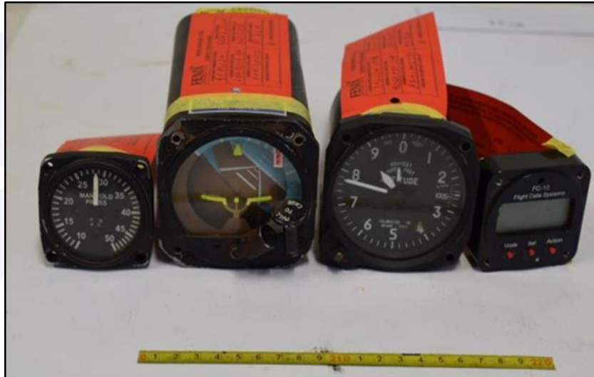
Figure 6 - View of the Manifold Indicator, Indicator Altitude Gyro, Altimeter and Fuel Computer instruments. |
