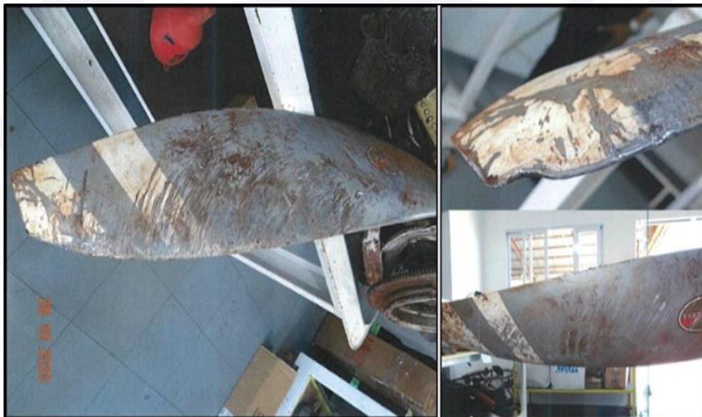
Figure 4 - (LE) View of the transverse scratches on the blade.
