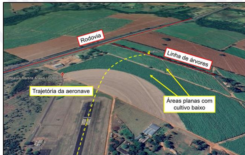
Figure 21 - Aircraft trajectory to the point of impact, highlighting the areas in which an emergency landing could have been made.
