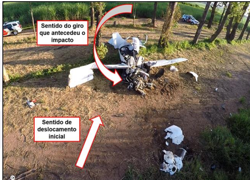
Figure 8 - General view of the wreckage and of the impact dynamic.
